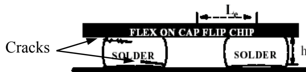
Figure 2.18 A first-order estimation of the fatigue life of solder joints.
