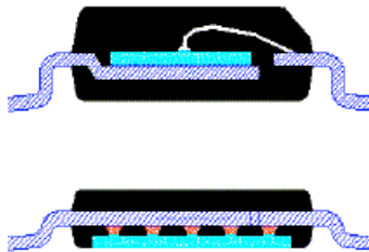
Figure 2.10 Conventional wire bond SOIC-8 (top) and the FLMP SOIC-8 package (bottom) (reprinted with permission of Rajeev Joshi, Fairchild Semiconductor).
