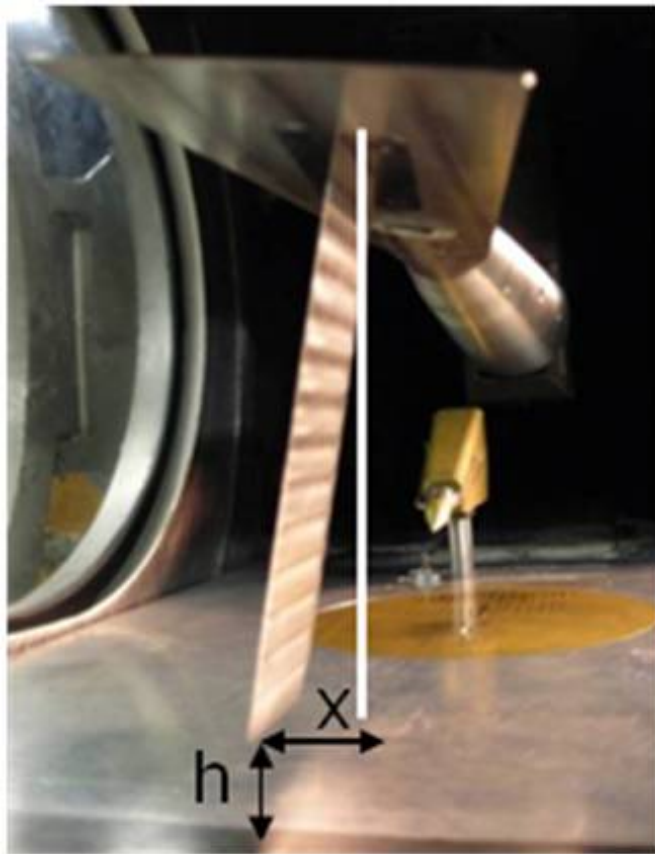
Figure 7.10: Wing tip position. The adopted reference system
