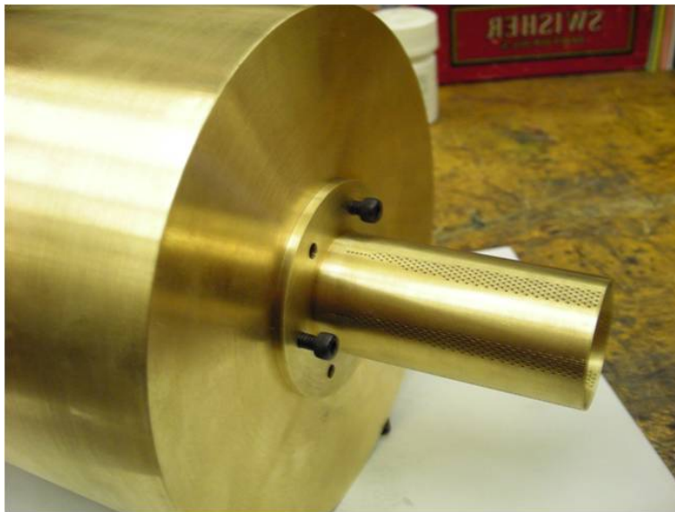
Figure B.5: Picture of the plenum and perforated nozzle assembly
