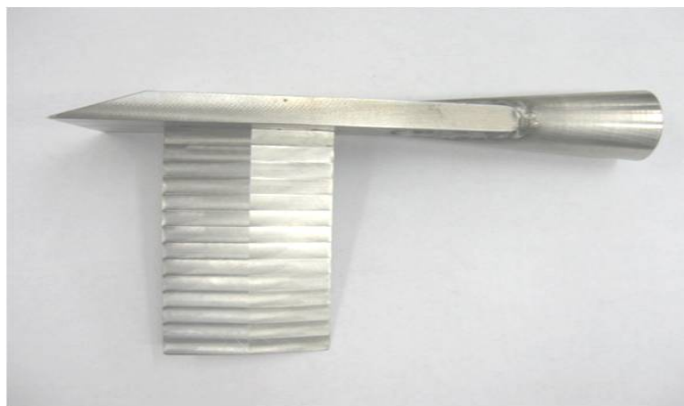
Figure 2.12: Picture of the vortex generator outside the wind tunnel
