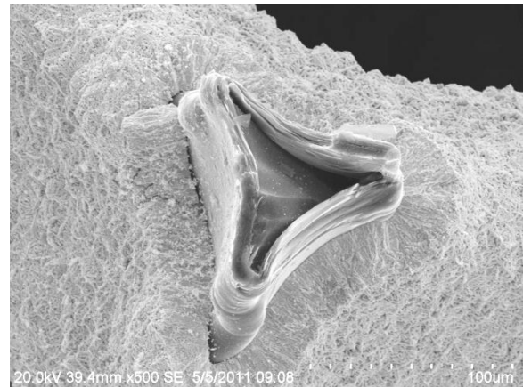
Figure 36.(left) Cross-section of a strut in a 45 ppi TaC/PyC/RVC foam
