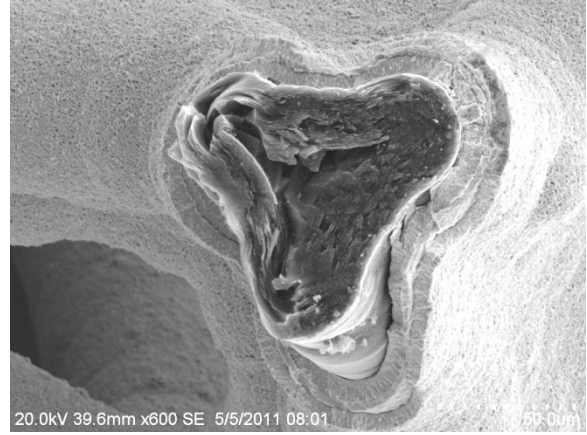
Figure 38.(left) Cross-section of a strut in a 100 ppi TaC/PyC/RVC Type A foam Figure 39.(right) Cross-section of a strut in a 100 ppi TaC/PyC/RVC Type B foam
