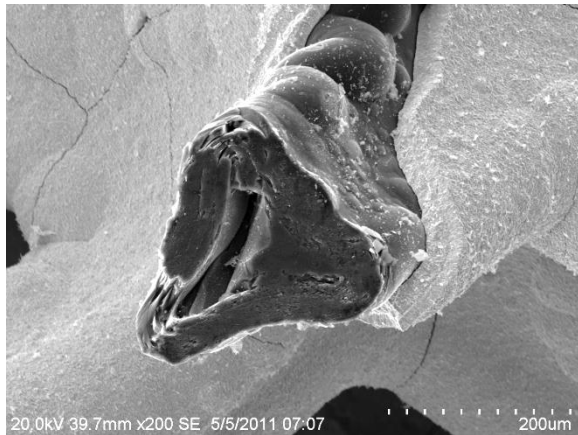
Figure 36.(left) Cross-section of a strut in a 45 ppi TaC/PyC/RVC foam
