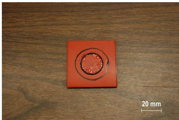
Figure 20.(left) Image of the specimen support platform that was used for flexural vibration measurements. Figure 21.(right) Image of the specimen support platform that was used for anti-flexural vibration measurements.
