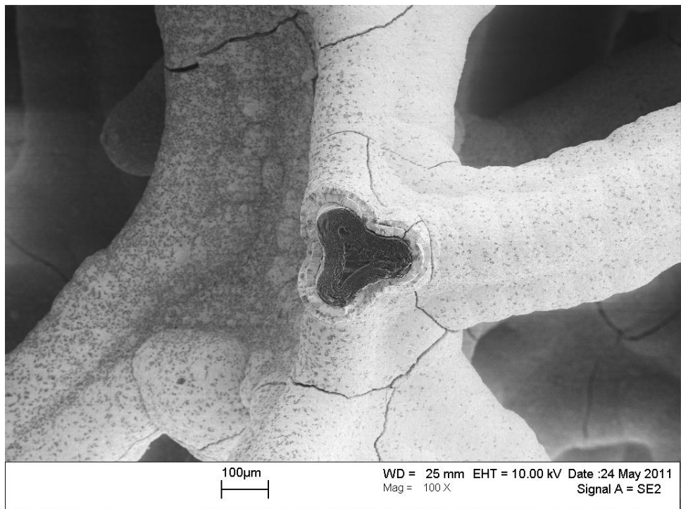
Figure 188. SEM micrograph of the microstructure of a 45 ppi TaC/PyC/RVC foam specimen after thermal cycling.
