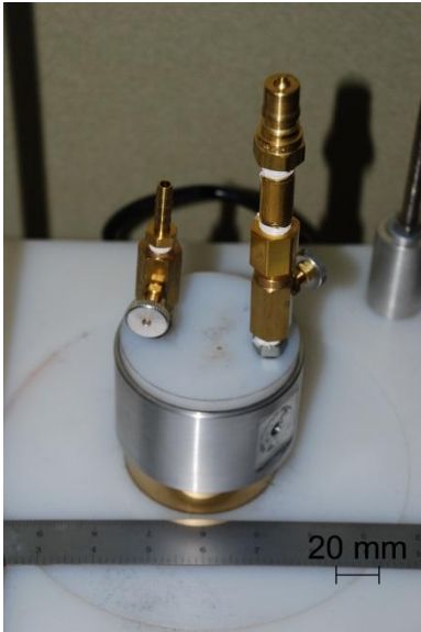
Figure 8.(left) Container for infiltrating foam under argon and vacuum. Figure 9.(right) Container for infiltrating foam with top removed
