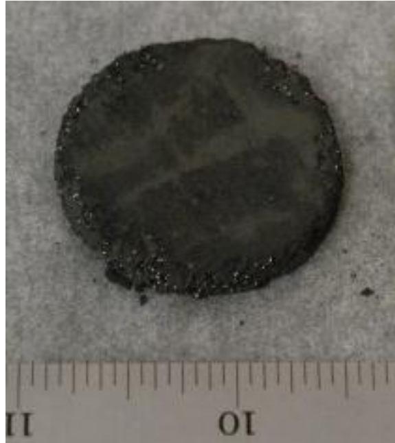
Figure 104. Infiltrated 45 ppi RVC foam prior to sintering
