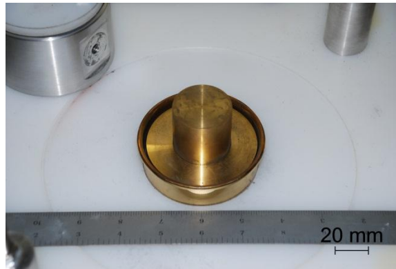
Figure 11. Image of brass punch within brass die, both of which are within the brass dish.
