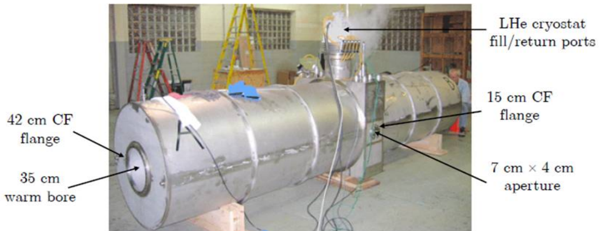
Figure 2.9: Photograph of the front face of the SCS magnet. The UCN enter the magnet from the 7cmX4cm aperture of the magnet. A rectangular hole was chosen to maximize the cross sectional area of the UCN guide feeding the decay trap, while still maintaining the required magnetic field uniformity. Figure used with permission from Brad Plaster (2010) [140].
