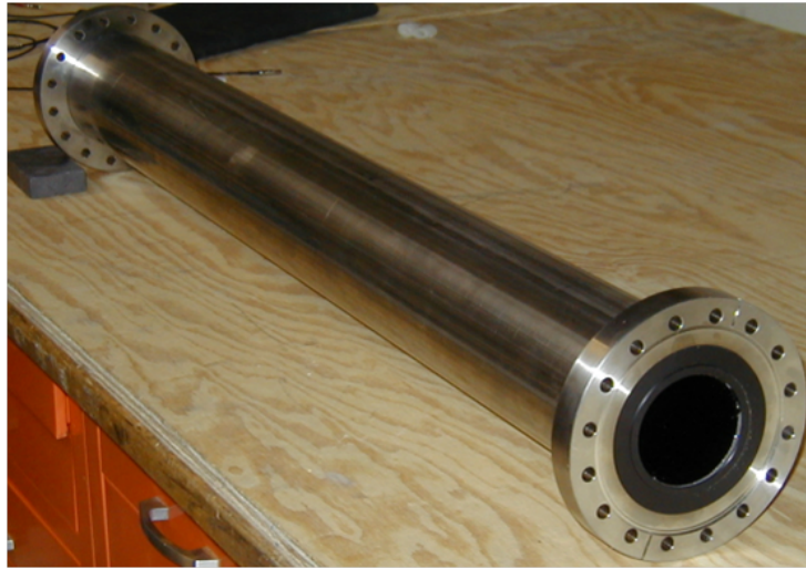
Figure 2.18: Stainless steel vacuum guide jacket used to provide the vacuum for the DLC quartz UCNA beamline. In the picture an acetal coupler is used to hold the guide. These were later replaced with copper versions. Figure used with permission from Mark Makela (2010) [111].
