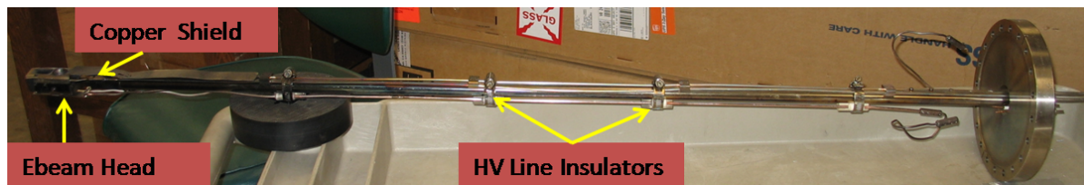
(b) Modified tube coating ebeam to address HV arcing and differential heating issues. The copper shield prevents stray electrons from bombarding the water lines and support rod
