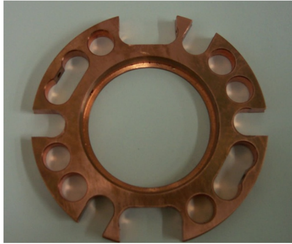
Figure 2.19: Example copper coupler used to hold the quartz guides. This particular coupler has two extra wide slots to accommodate water and electrical lines used by the RF spin flipper.
