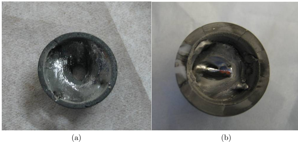
Figure 3.18: Comparison of the nickel melts in graphite and alumina crucibles after several ebeam deposition runs. (a) Hole drilled through the ^{58}\text{Ni} and graphite crucible. Notice the more crystalline structure indicating \text{Ni}_3\text{C} carbide formation. (b) ^{58}\text{Ni} in an alumina crucible after several depositions. The nickel does not alloy with the alumina, however the alumina crucible does eventually crack from thermal stresses during the deposition process.
