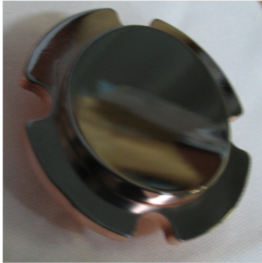
Figure 7.19: Photograph of the 7-30-09 DLC coated Plug. The plug was placed such that the “plasma shoots” provided most of the coating. The thickness ended up being > 262 nm.
