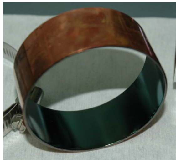
(b) Close up of the DLC coating on the copper tube
