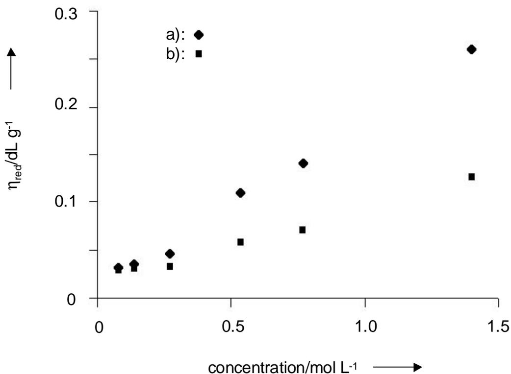
**Figure 11.8.** Reduced viscosity as a function of concentration (solutions in acetone at 22°C) a) **5** and b) **1b** and **6** (1:1).
