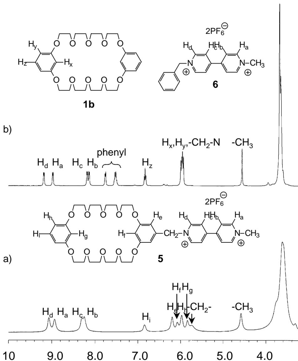
**Figure 11.6.** The  $^1\text{H}$  NMR spectra of a) **5** at 2.0 M and b) **1b** and **6** (2.0/2.0 M) (400 MHz, acetone- $d_6$ , 22°C).
