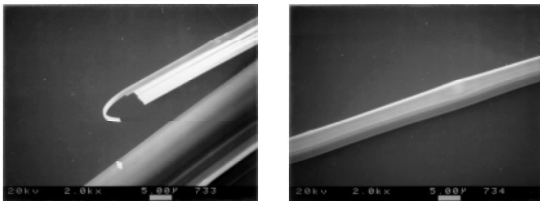
**Figure 11.10.** Longitudinal views of scanning electron micrographs of a fiber pulled from a concentrated acetone solution of **3** (>2.0 M).
