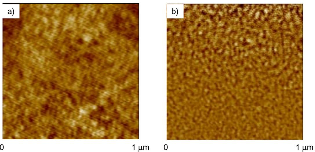
**Figure 11.11.** The AFM images of a fiber pulled from a concentrated acetone solution of **3** (>2.0 M) a) height and b) phase.
