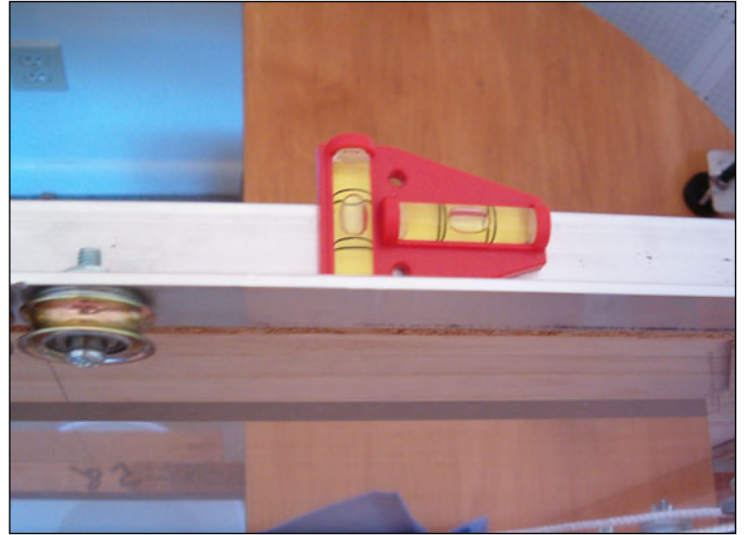
Figure Z8. Checking for level of the truss tester.
