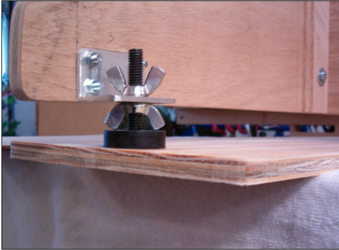
Figure Z7. Adjustable feet so truss tester can be leveled.
