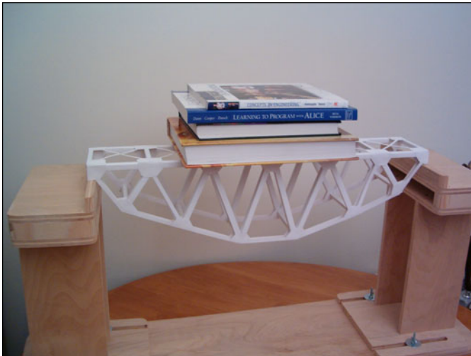
Figure C5. Card stock bridge with static load applied.
