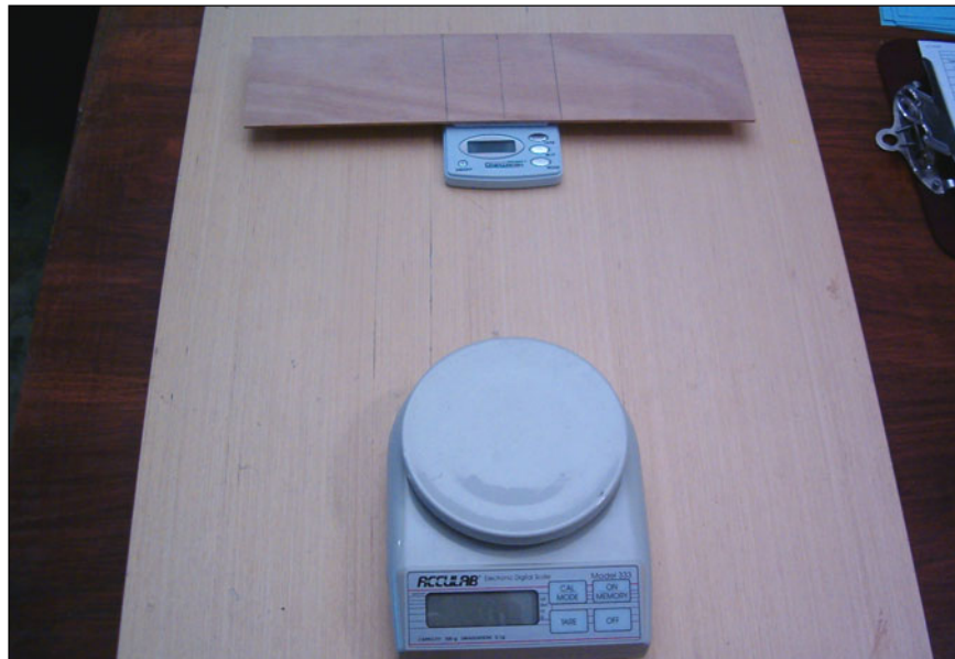
Figure Z16. The mass of each truss was measured with two scales.
