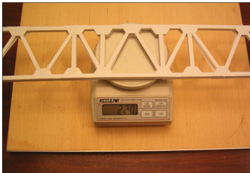
Figure Z17. Trusses were lined up with the center joint on the scales.
