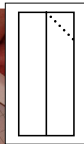
2. Rotate tube away from you 90° and draw a line straight across.
