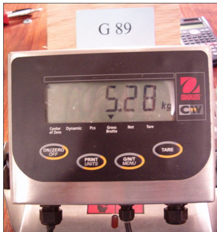
Figure Z15. Photos were made for each mass at which the truss failed.
