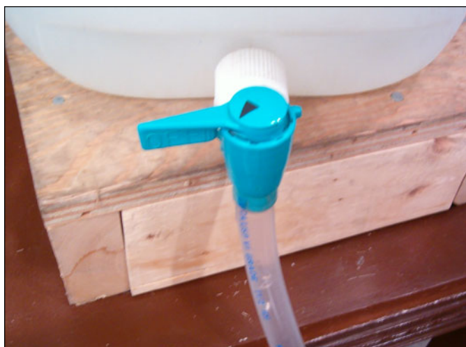
Figure Z12. A notch was placed on the water valve.
