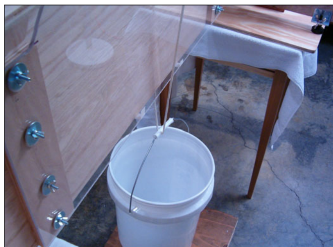
Figure Z5. Bucket for holding water to apply the load.
