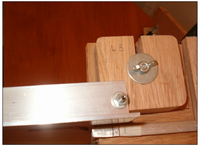
Figure Z10. Track was made parallel to the truss.
