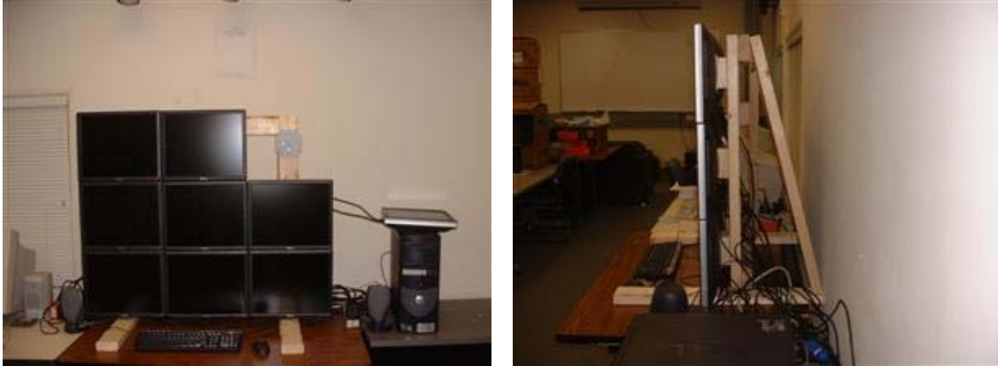
Figure 13. View of the nine-monitor display stand from the front and side.
