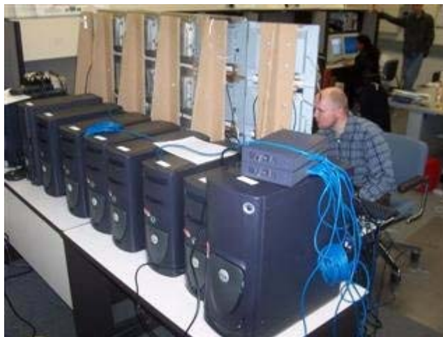
Figure 17. Shot of the back of the display cluster showing computers driving the display.
