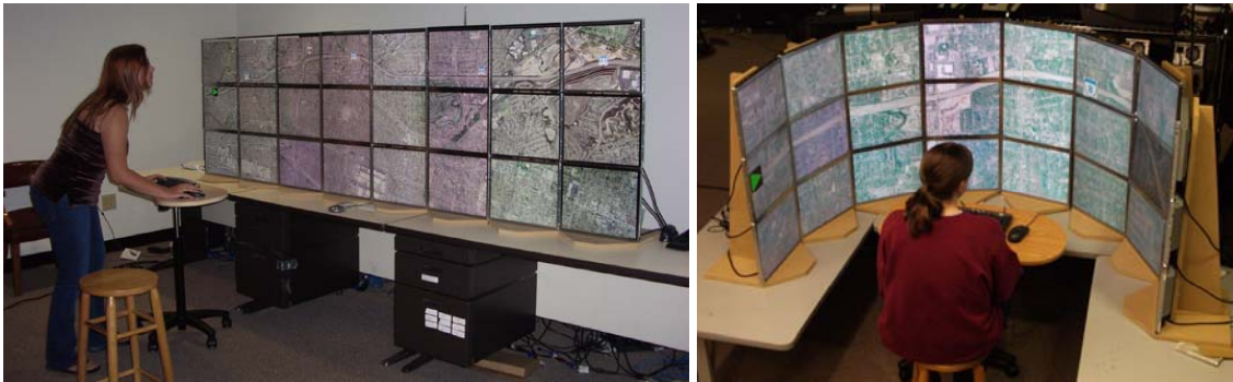
Figure 40. Twenty-four monitor flat configuration (left) and twenty-four monitor curved configuration (right).
