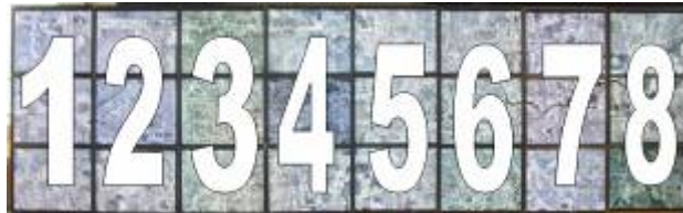
Figure 45. Image showing how the display was artificially separated into different columns. The total resolution of the display is 10240 X 3072. The physical dimensions of the display were roughly 9 feet (2.7 m) by 3.5 feet (1 m).
