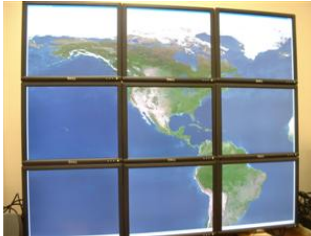
Figure 22. The nine-monitor tiled configuration. The total resolution is 3840x3072 (11,796,480 pixels).
