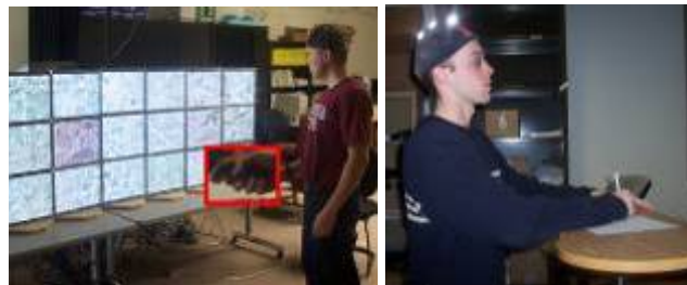
Figure 46. a) Image showing a participant using the gyro mouse with the display. The gyro mouse is enlarged in the red square. b) An image showing the hat used to track users' position.
