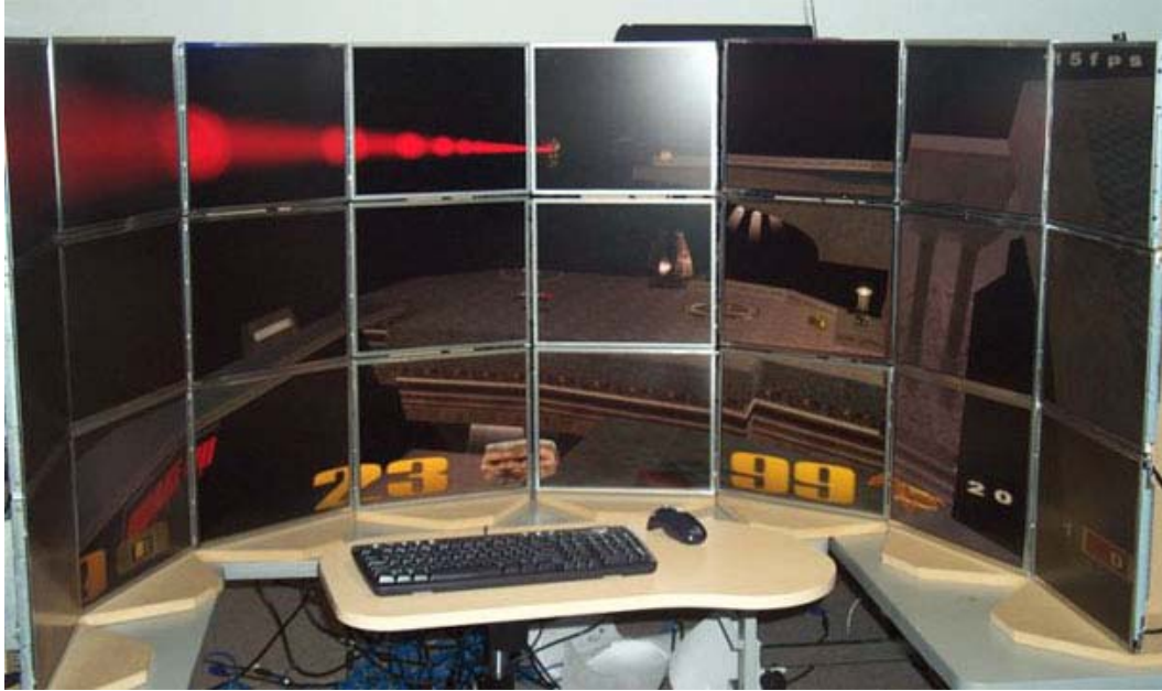
Figure 20. Quake 3 running at 10240x3072 resolution at 15-30 FPS. This is possible due to Chromium.
