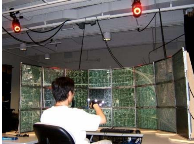
Figure 18. Example of a user interacting with the curved display using the VICON system as an input device.
