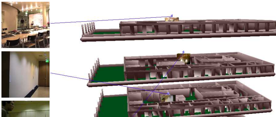
Figure 4-3: Associated Video. Callout lines are used to show association.
