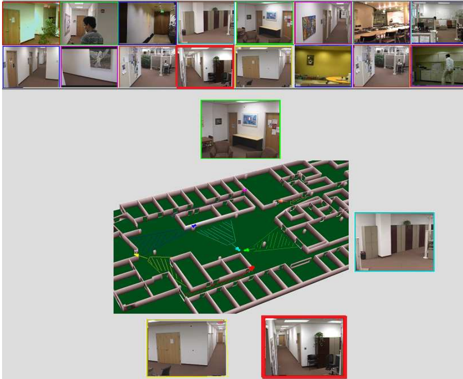
Figure 8-2: Prototype for overview navigation interface. All the cameras and their coverage area should be shown in the 3D model. The red camera is selected and highlighted.
