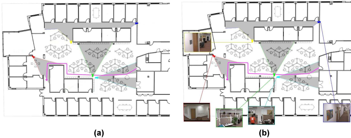
Figure 7-1: Dynamic Path Visualization Prototypes used in the formal experiment. The path dynamically shows the target person's trajectory from his first appearance in a video to the current moment. (a) Dynamic Path Visualization without videos. (b) Dynamic Path Visualization with videos.
