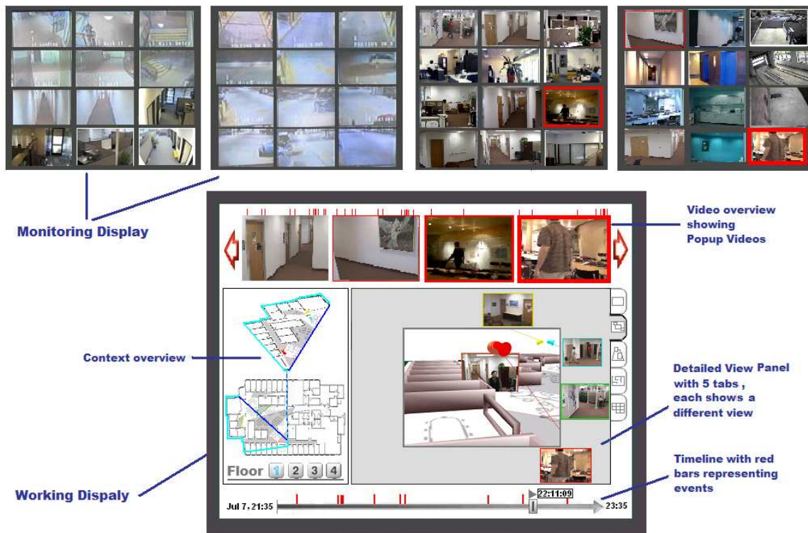
Figure 9-2: Interface for the new system, which contains a monitoring display and a working display. The working display contains four areas: The area on top is the Popup Videos area. At bottom is the Timeline. Of the two areas in the middle, the right is the Detailed View, which contains five tabbed panels. The left area is called Context Overview.
