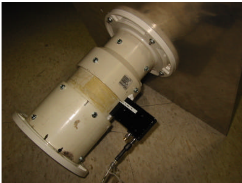
(b) A hardware test model using the 1-port measurement method.
