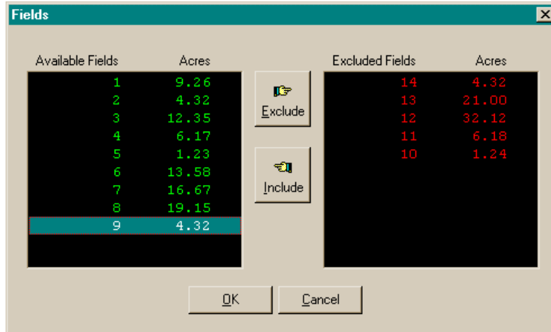
Figure 3-13 Active Fields Editor window. Fields from the left list can be removed from planning and put into the excluded list on the right.
