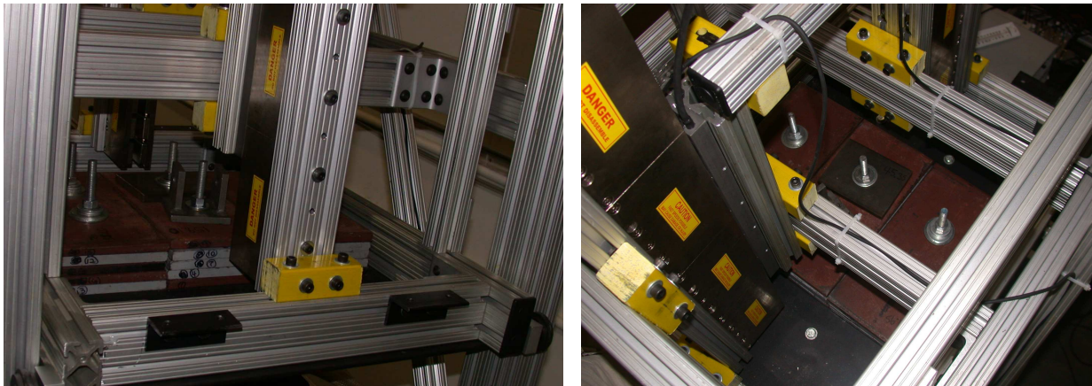
Figure 6.12: An additional 155 lb (70.307 kg) of weights as part of m_1
