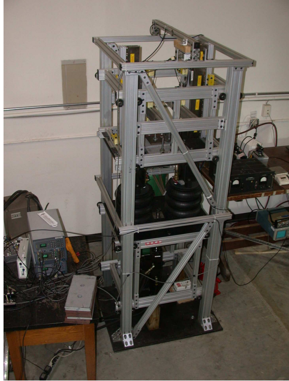
Figure 6.10: The mechanical oscillator configured for testing a distribution of masses for m_1
