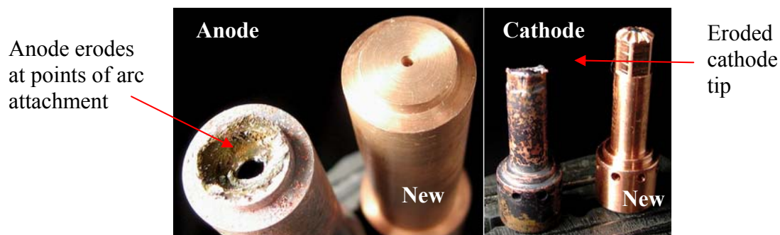
Figure 1.22. Erosion in the anode (left) and cathode (right), compared to new electrodes. On the left, the uniform erosion of the anode about the orifice indicates that the arc is swirling and not attaching only to one side of the anode, despite the supersonic crossflow.
