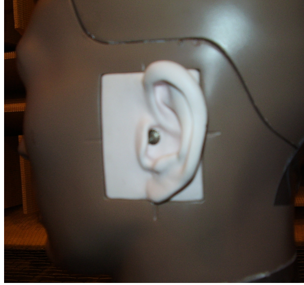
Figure 7.1 Left pinna insert in KEMAR manikin head.
