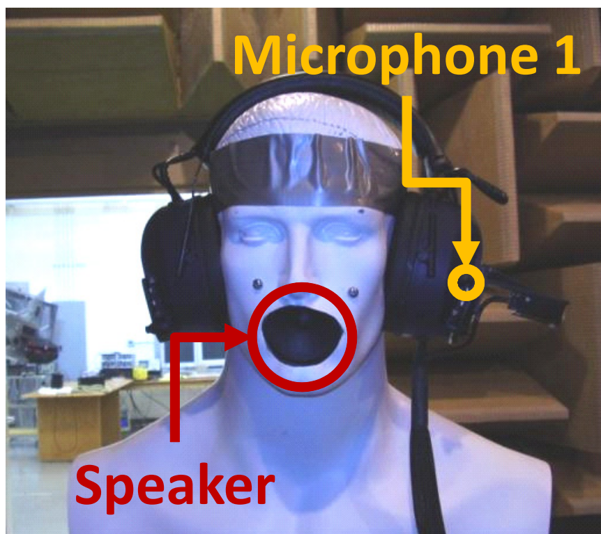
Figure 6.4 Manikin wearing headset array with speaker mounted in mouth(red).
