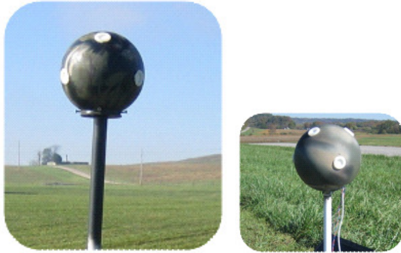
Figure 3.6 Spherical diffracting arrays used for experimental data collection and system testing.
