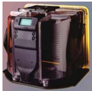
Figure5.1: A front opening unified pod (FOUP)
