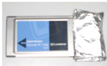
Figure 4.2 Antenna portion of the wireless PC Card wrapped with aluminum foil “attenuator.”
