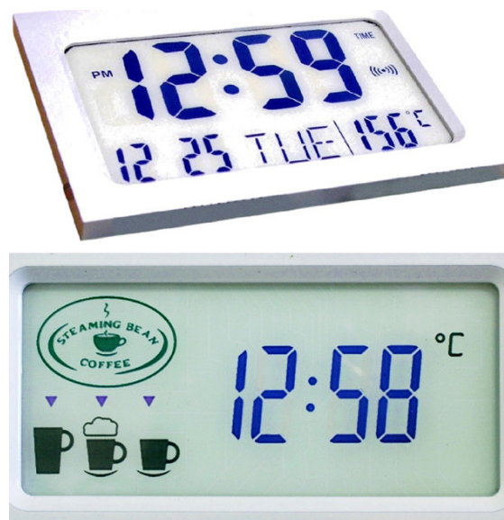
Figure 2.22 Nanochromics displays. [Reprinted from N. Vlachopoulos, J. Nissfolk, M. Moller, A. Briancon, D. Corr, M. Ryan, A. Hagfeldt, Electrochemical aspects of display technology based on nanostructured titanium dioxide with attached viologen chromophores, Electrochim. Acta , 2008 , 53, 4065 with permission from Elsevier] 159
