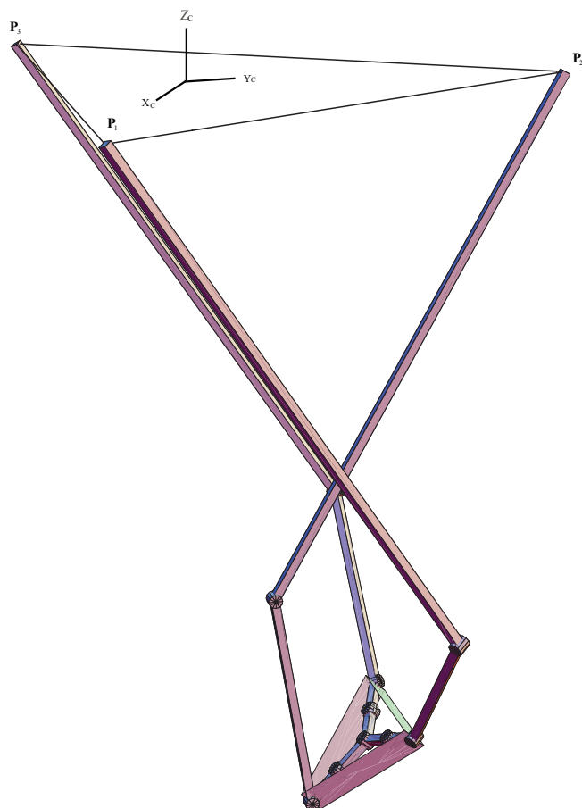
FIG.3.6 FORWARD DISPLACEMENT SOLUTION 6
