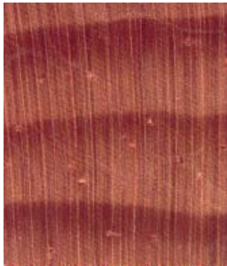
Figure 2. 2 Red pine ( P.resinosa ) cross section structure 20× (Hoadley 1980).
