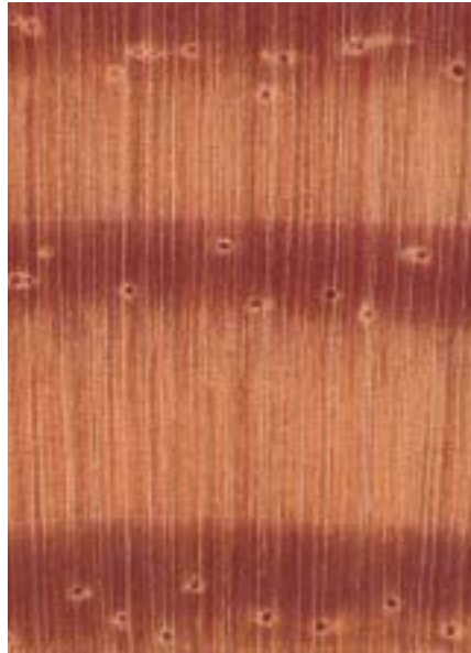
Figure 2. 1 Southern yellow pine ( Pinus spp.) cross section structure 20× (Hoadley 1980).
