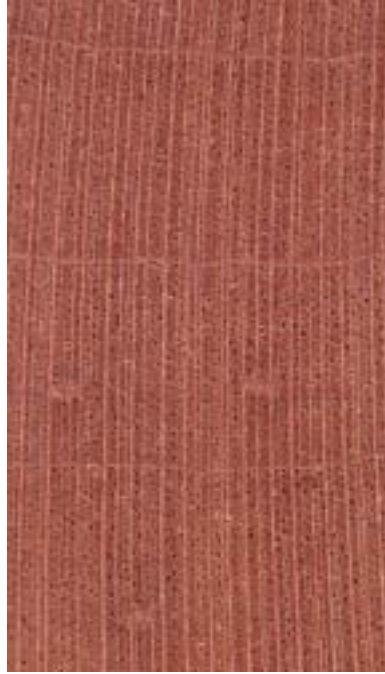
Figure 2. 3 Red maple ( Acer rubrum ) cross section structure 20× (Hoadley 1980).
