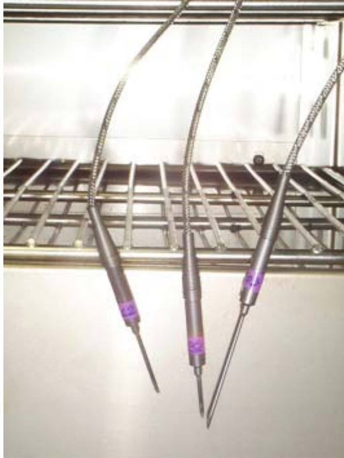
Figure 3. 17 Hypodermic thermocouples used in the test with 1/16" diameter of the probe. The temperature was measured only at the tip of the probes.
