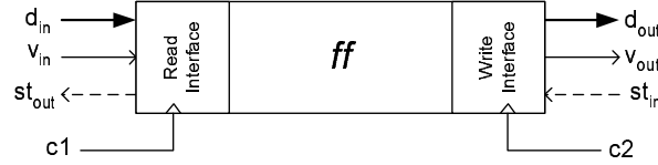
Figure 8.7: Block Diagram of Interface FIFO
