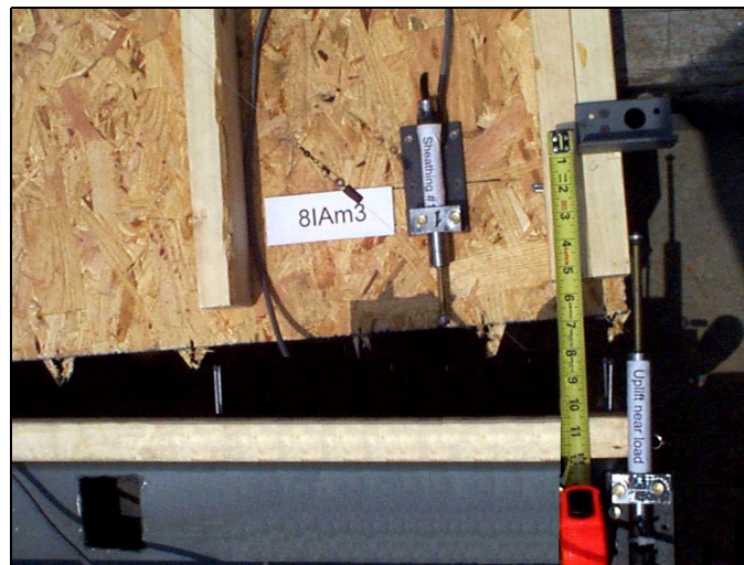
Figure 5. 25. Failure mode of 08IAM wall with 10-mm edge distance.
