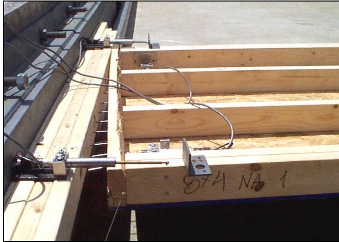
Figure 5. 40. Wall attached with 12 nails in one row.
