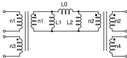
Figure 5.14 Circuit model of general integrated magnetic structure
