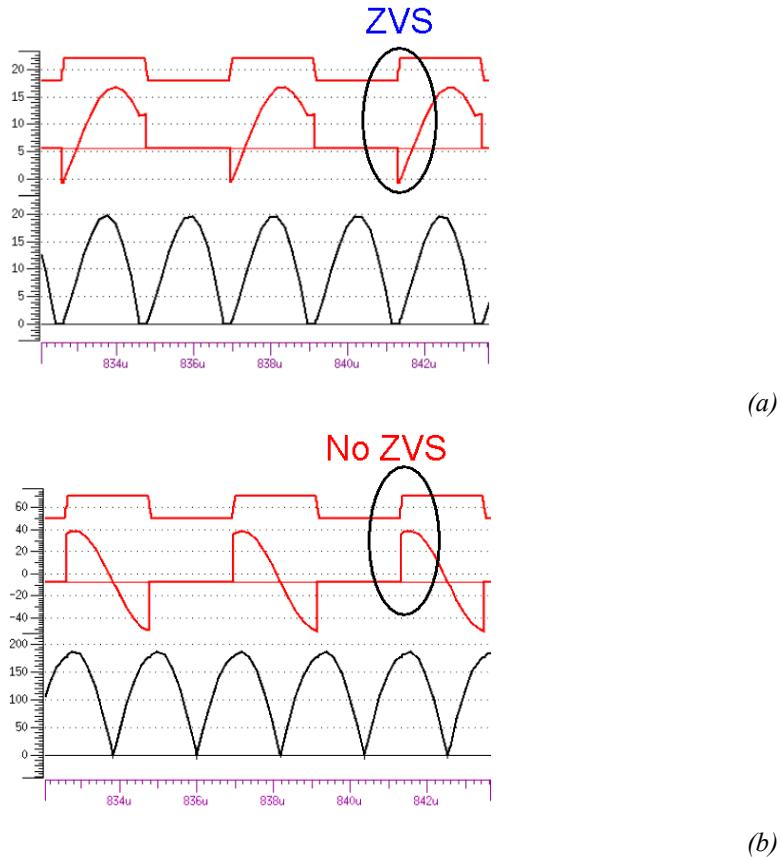
Figure 5.24 Simulation waveforms of LLC resonant converter at (a) normal operation, and (b) short circuit operation
