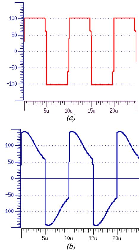
Figure 5.8 Voltage stress of output diodes D1 D2 (a): desired structure (b) real transformer
