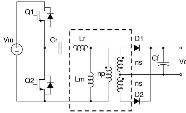
Figure 5.1 Magnetic structure for LLC resonant converter
