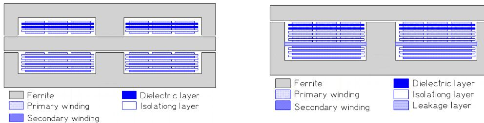
Figure 5.49 Two passive IPEM structures for LLC resonant converter
