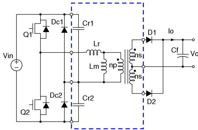
Figure 5.46 LLC resonant converter with splitting resonant cap and clamping diodes
