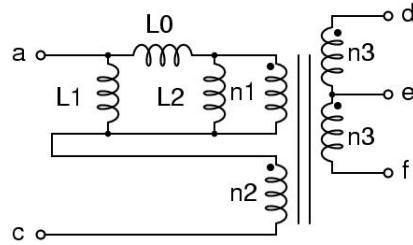
Figure 5.17 Electrical model of connecting dot-marked terminal with unmarked terminal
