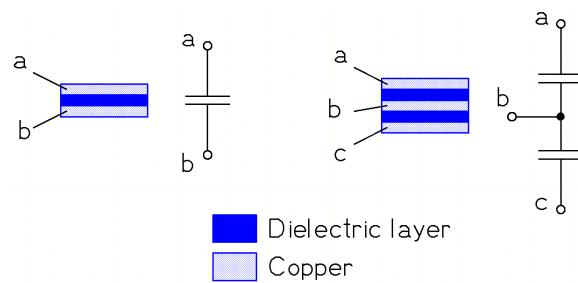
Figure 5.48 Capacitor integration for LLC resonant converter
