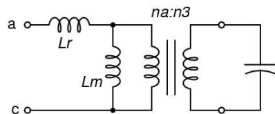
Figure 5.19 Equivalent-circuit for mode (a)
