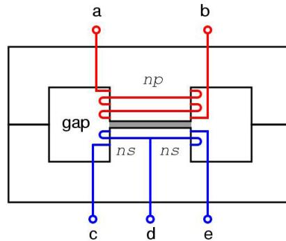
Figure 5.5 Structure with real transformer
