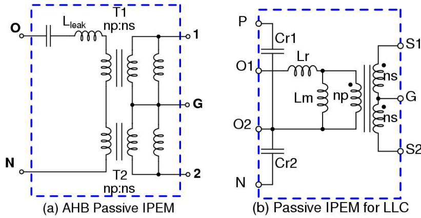
Figure 5.47 Schematics of passive IPEMs for AHB and LLC r converter
