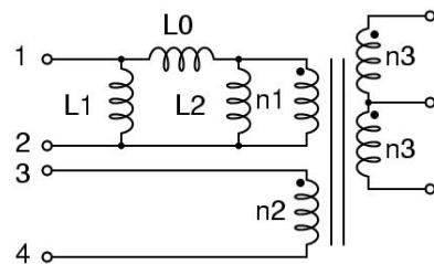
Figure 5.16 Electrical circuit model of integrated magnetic structure B
