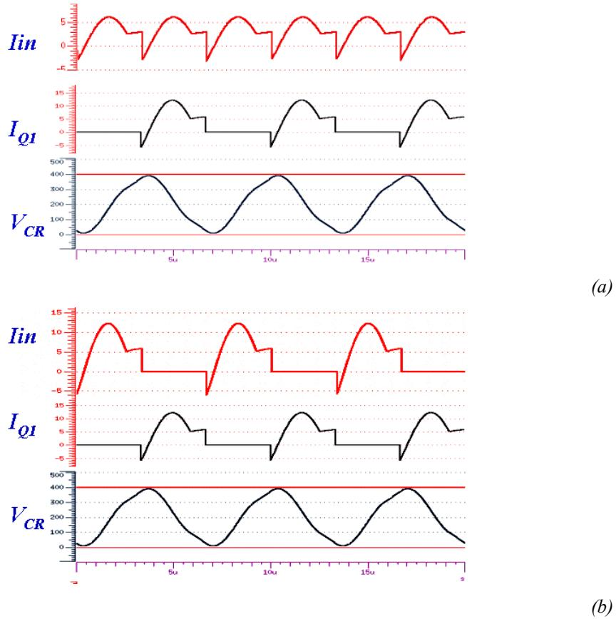
Figure 5.39 Simulation waveforms for two LLC resonant converter topologies: (a) original LLC converter and (b) clamped LLC converter
