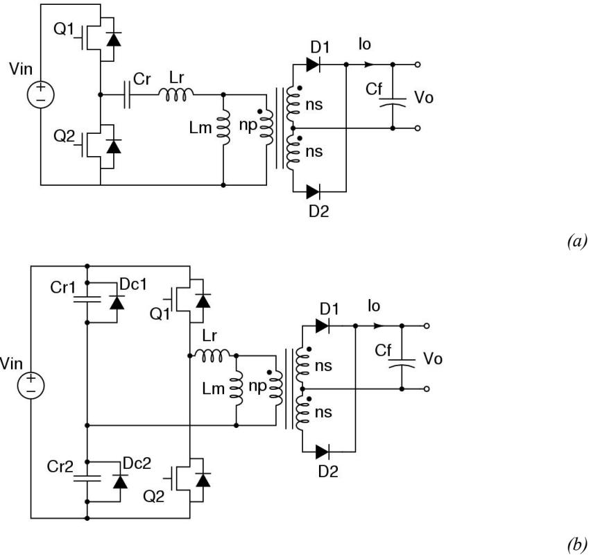
Figure 5.38 Two LLC resonant converter topologies: (a) Original LLC converter and (b) proposed clamped LLC converter
