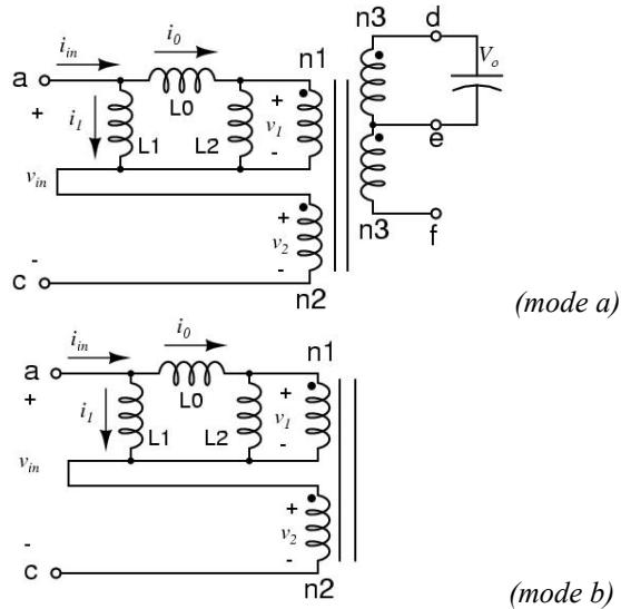
Figure 5.18 Two operation modes for LLC resonant converter
