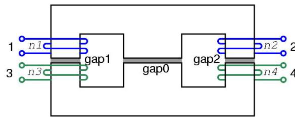
Figure 5.12 general magnetic structures for Integrated magnetic
