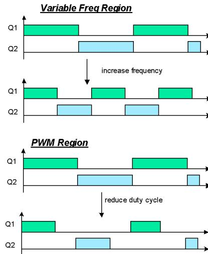
Figure 5.33 Control Method of Variable freq + PWM control
