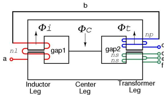
Figure 5.9 Integrated Magnetic Designs A
