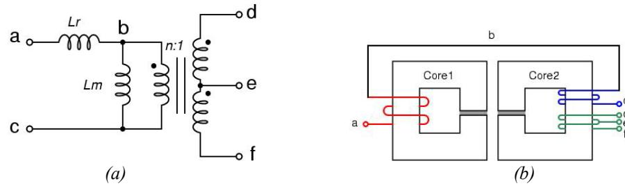
Figure 5.2 Discrete magnetic design (a) schematic (b) physical structure
