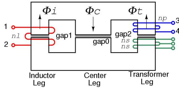
Figure 5.15 Integrated Magnetic Designs B
