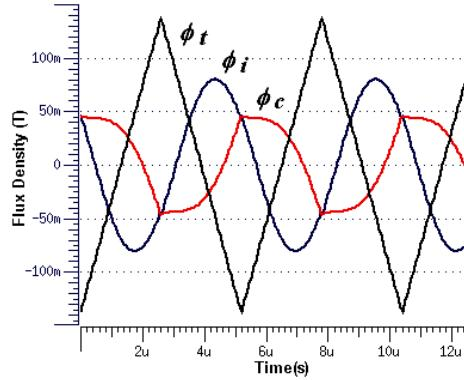
Figure 5.10 Flux density simulation result for Design A
