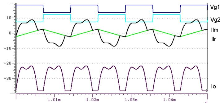
Figure 7.3 Simulation waveform of LLC resonant converter with passive current shaping
