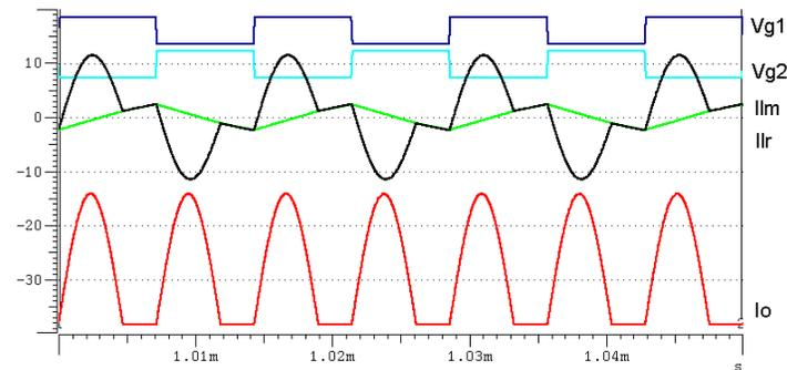
Figure 7.2 Simulation waveform of LLC resonant converter
