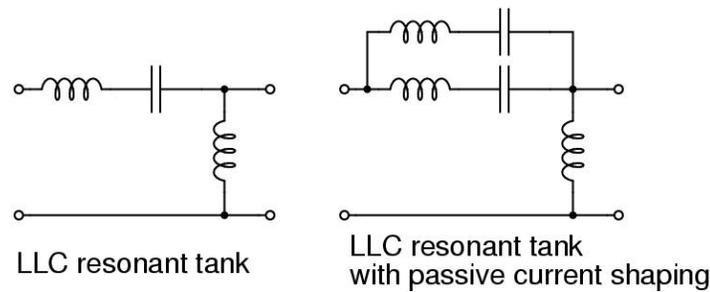
Figure 7.1 LLC resonant tank and LLC resonant tank with passive current shaping
