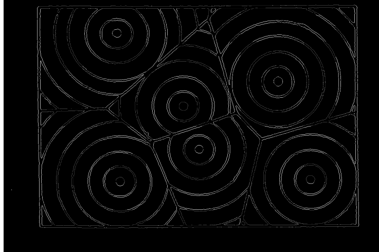
Figure 2.4 Schematic depicting spherulitic impingement and radial growth rings. 52
