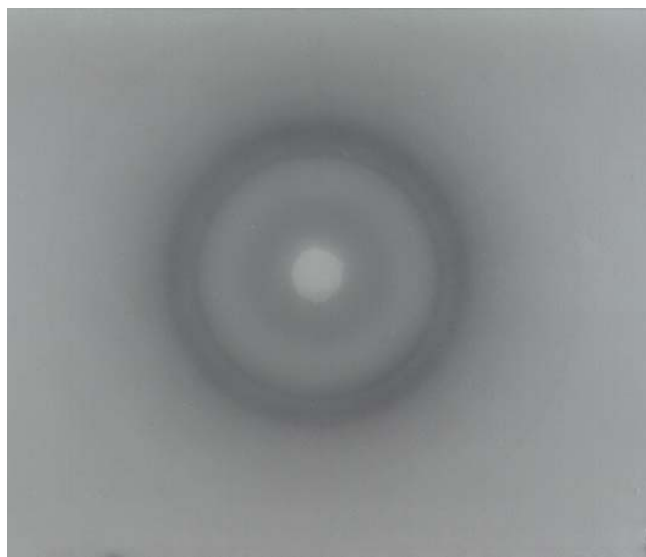
Figure VII.3 WAXS pattern of the segmented PAES containing 50% BP and 50% DHTP.
