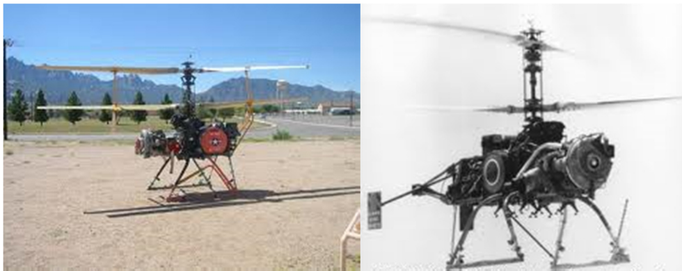
Figure 5: The US Navy Drone Anti-Submarine Helicopter (DASH). Public Domain
