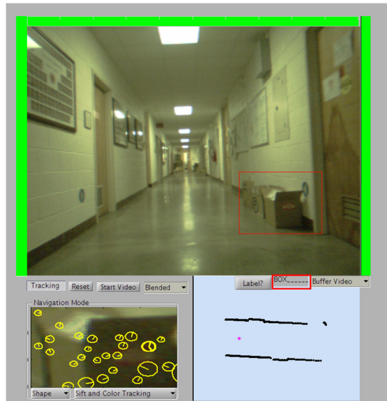
Figure 88: Dominant Maturity Recognition as seen through the RobiSEND GUI. The object model features have been recognized as a previous object model called "BOX". This is displayed to the user as shown with the red highlight in the image.
