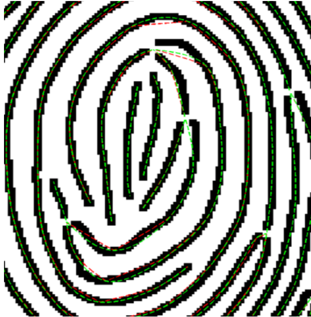
Figure 4-4: Region surrounding core point in a binary fingerprint image with cubic spline fit (green) and linear approximation (red) to ridges.
