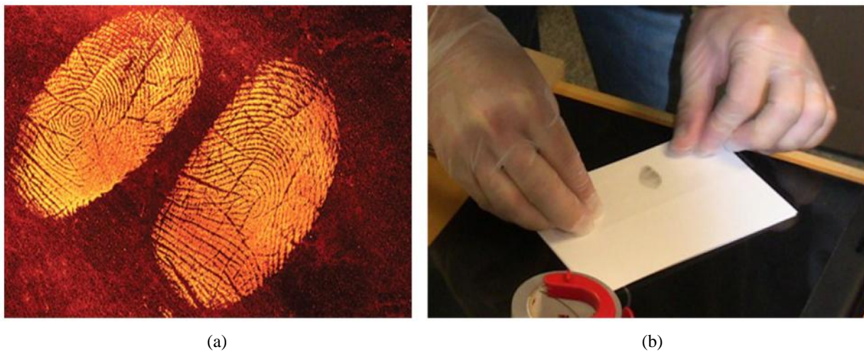
Figure 1-9: Examples of (a) fingerprint dusted with orange powder and photographed with blue cut-off filter (reproduced from [2]) and (b) latent print being transferred with adhesive method.
