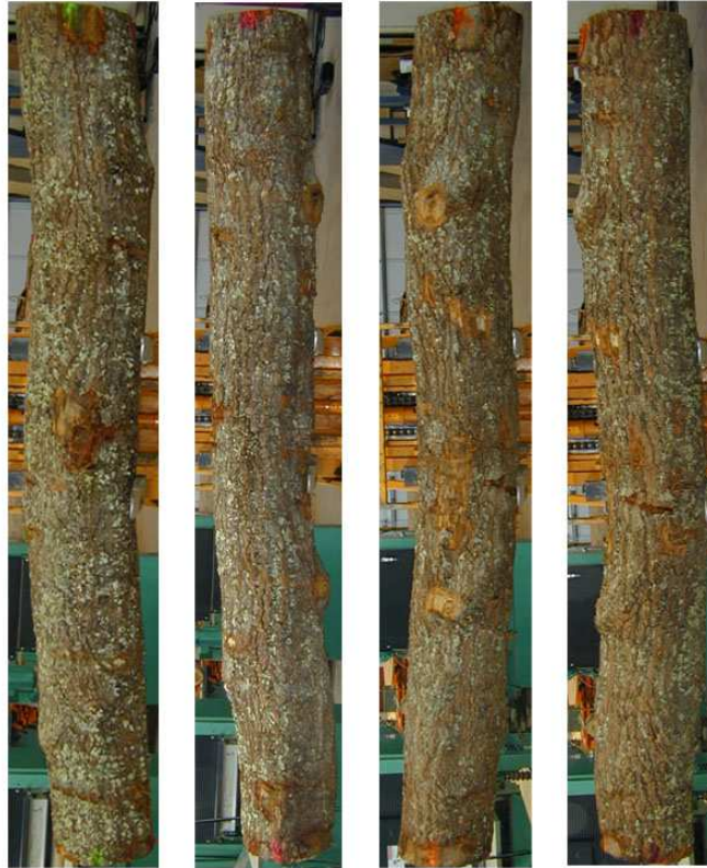
Figure 6.4: Four digital intensity image of a log sample at 90^\circ per side. These images are used in part to determine the correctness of the machine generated defective regions.
