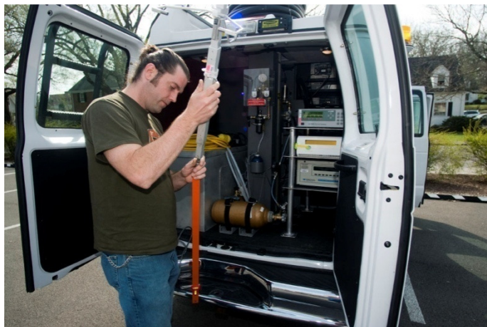
Figure 4. Rear view of FLAME measurement platform showing sensor equipment configuration. Relaxed eddy accumulation system is also located in the rear of the van and is shown in Figure 3.
