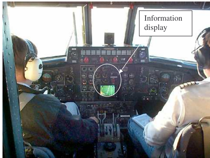
Figure 2-1. Aircraft position, velocity, weather, traffic, advisory information display in the cockpit using the avionic system [Mood03]
