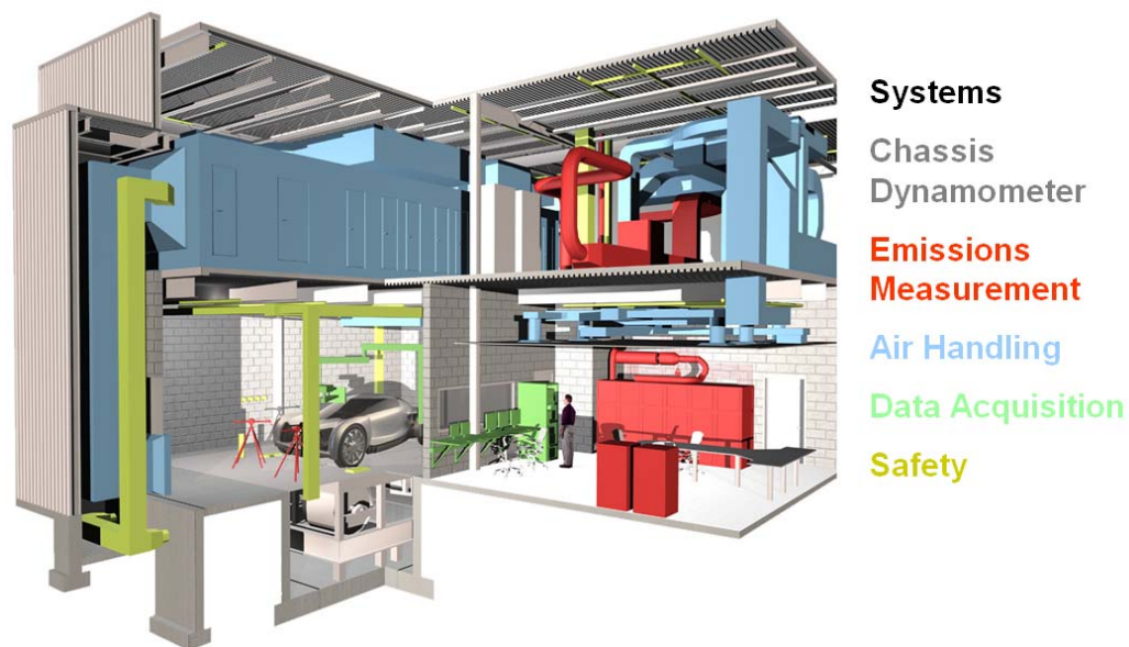
Figure A1-1: Illustration of the Advanced Powertrain Research Facility infrastructure
