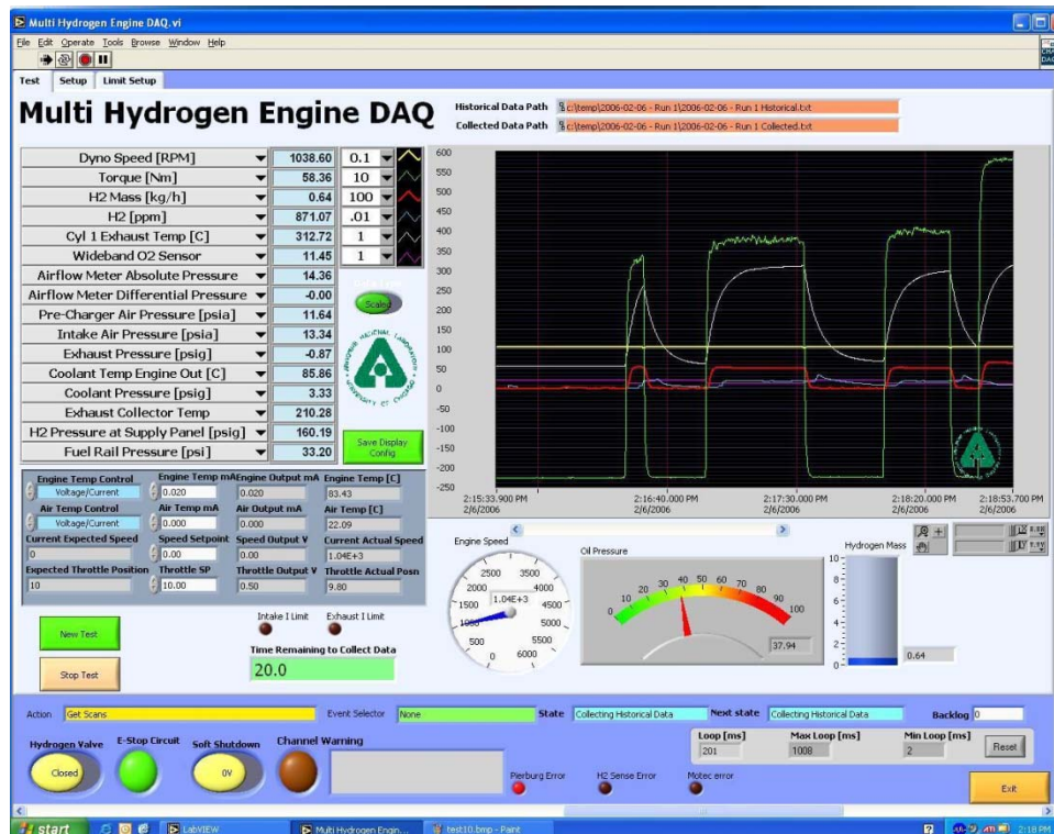
Figure 9-6: Screen shot of the data acquisition shows the first power produced by the engine
