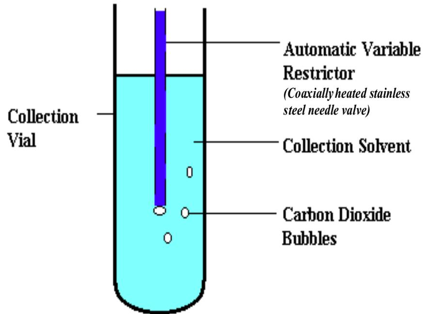
**Figure 1-1:** Schematic Representation of the Liquid Trapping Process
