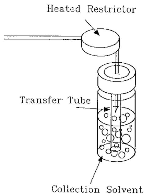
**Figure 1-2:** Schematic Representation of the Collection Systems Used in the Dionex Extractors
