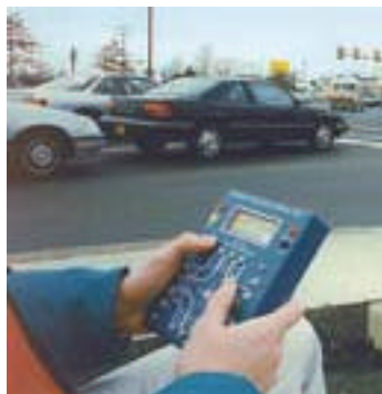
FIGURE 6.2 USE OF A TURNING MOVEMENT COUNTER AT AN INTERSECTION (Source: http://www.jamartech.com/prod02.htm )
