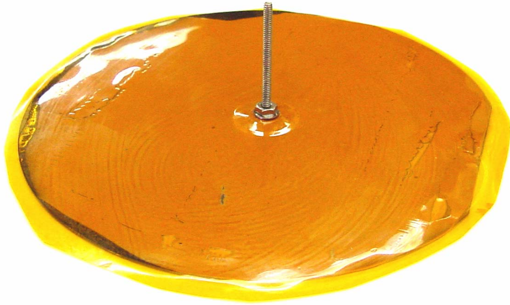
Figure 3-26 Photograph of L4 adhesive blister specimen.
