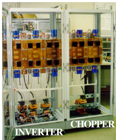
Figure 2.29. Experimental SMES PCS system.
