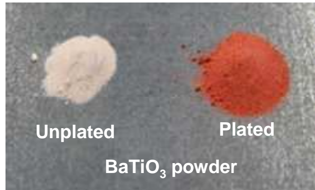
Figure 41. Unplated vs. electroless Cu plated BaTiO 3 reinforcement powder
