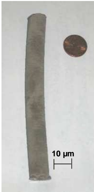
Figure 28. Electroformed nickel sample having 0v% BaTiO 3
