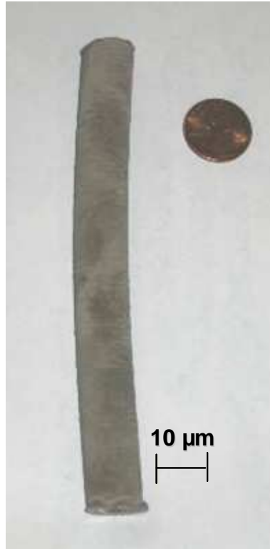
Figure 51. Electroformed Ni-BaTiO 3 composite rod after fabrication
