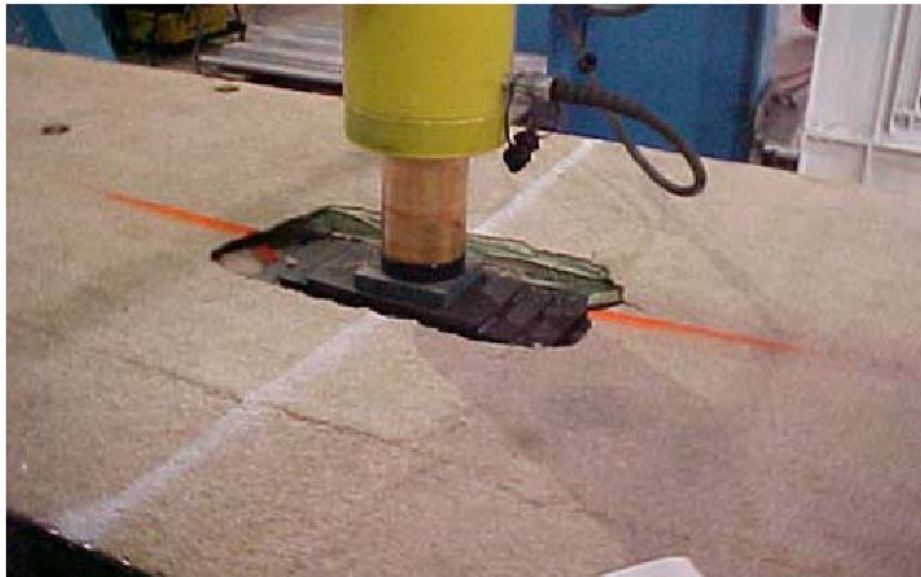
Figure 1.8 Punching failure using steel patch
