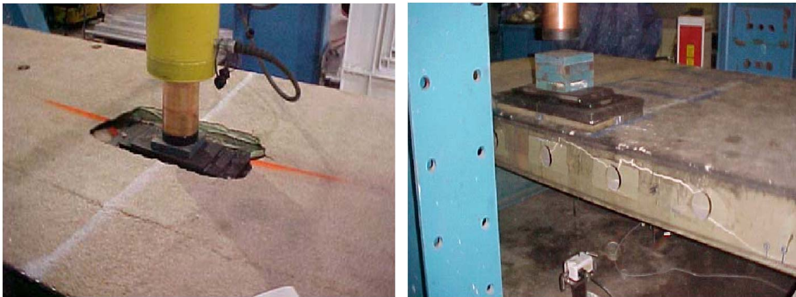
Figure 5.1 Failure of Deck A using steel loading patch [Temeles, 2001]
