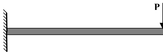
Figure 3.52 Cantilever Bending Beam
