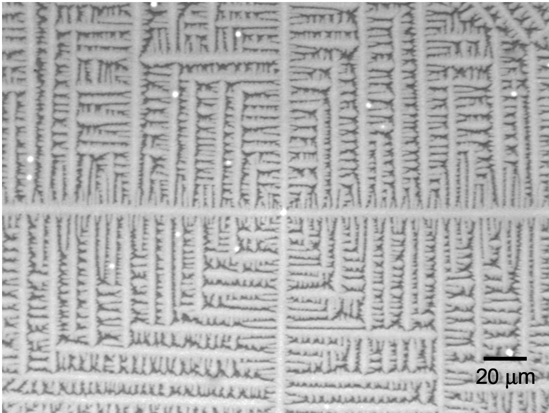
Figure 3.1 Example of a dendrite in a 30/70 PMMA7 sample crystallized at 37°C.
