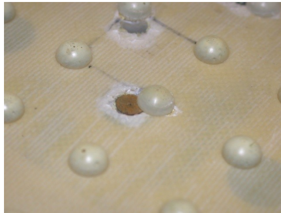
Figure 2-28. Detailed view of the wall pressure microphone configuration around a 3mm hemispherical element
