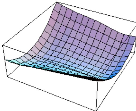
**Figure (6.5) : Predicted nominal imperfection profile for the second optimum design**
