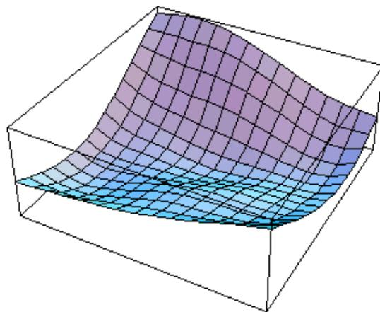
**Figure (6.7) : Predicted nominal imperfection profile for the new optimum design**
