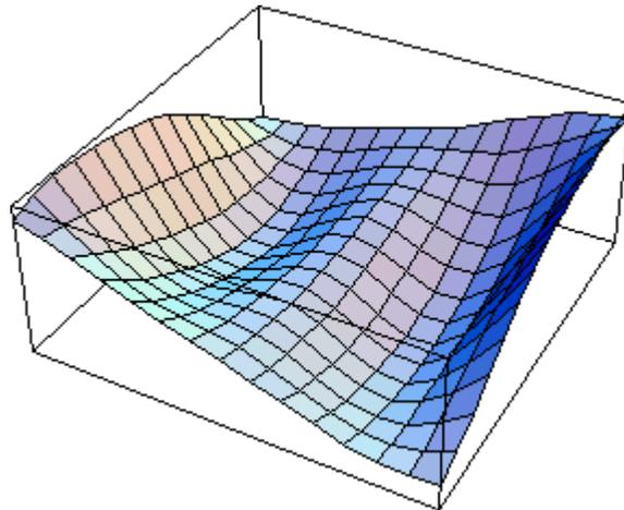
**Figure (6.3) : Imperfection profile used to initialize the design process**
