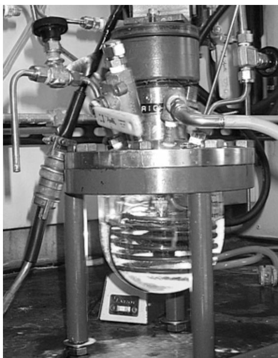
Figure 2.10: Anionic polymerization carried out in pressurized glass reactor system.
