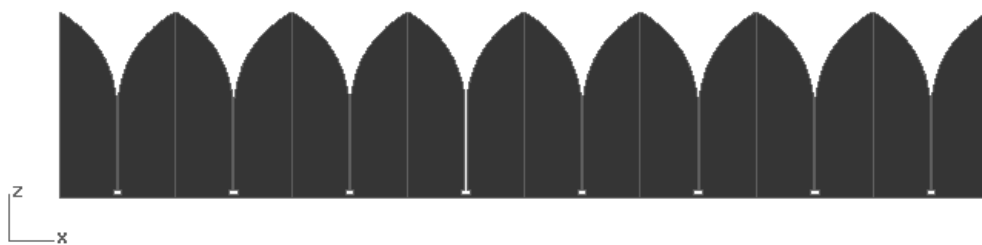
Figure 3-2 – Geometry of a 1x8 interconnected tapered slot array
