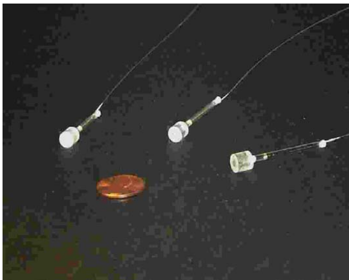
Figure 3.15 Photograph of three diaphragm-based sensor probes fabricated by inter-medium layer thermal bonding method
