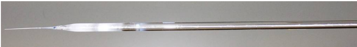
Figure 2.10- Preforms made by “Core-Suction” Technique using a tube Furnace (After cool down)
