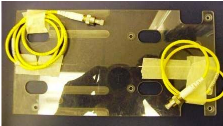
Figure 4.6- Photograph of the 5 cms MM2 glass fiber spliced to standard fiber pigtails
