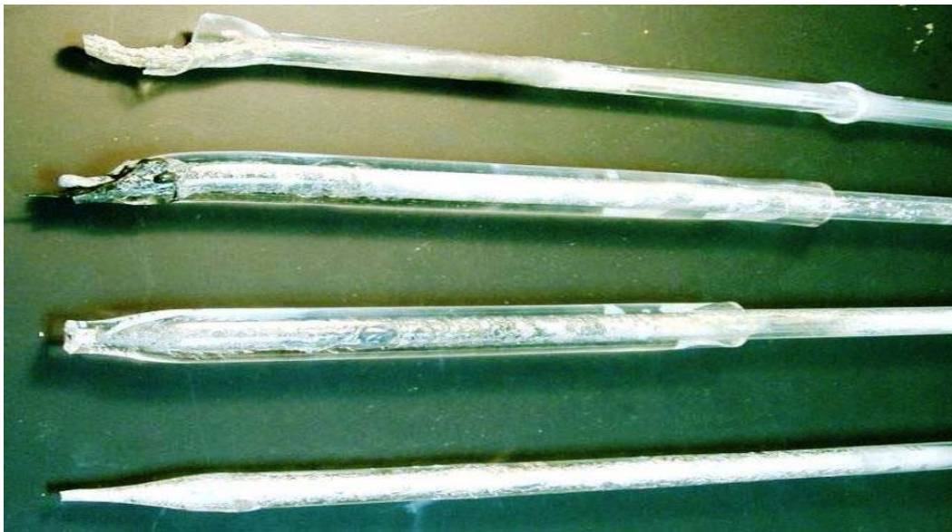
Figure 2.2- Crucible Preforms showing Blow-out, cracking and stresses on the interfaces
