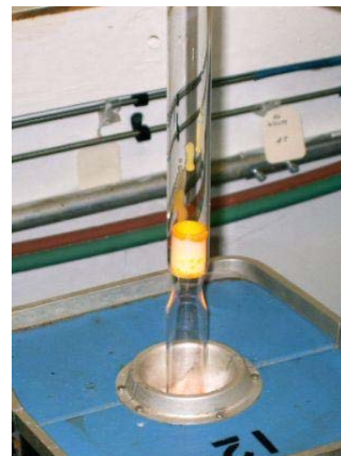
(e) Crucible inside the aligner with Molten Core Material
