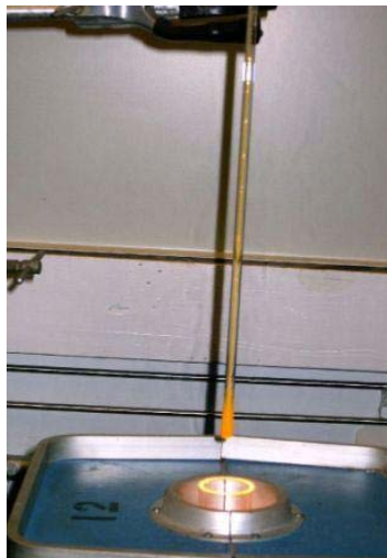
(d) Cladding Tube just after Suction of Core Material
