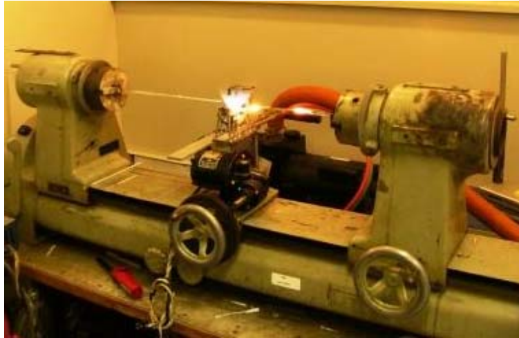
Figure 2.20- Horizontal Lathe Shrinking the Cladding Tube
