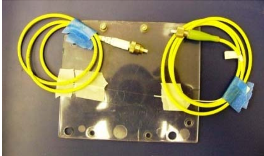
Figure 4.8- Photograph of 1 cm MM2 glass fiber spliced to standard fiber pigtailed
