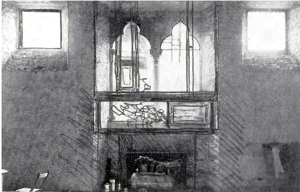
fig. 2.16 Carlo Scarpa Free hand ink drawing on photograph (1950s-'70s) Detail of a window towards the courtyard. Sketch of the new interior window moldings. © Castelvecchio Museum
