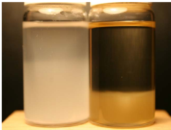
Figure 3.8 Ctrl in water (left) and Amd in toluene (right) three days after dispersion.
