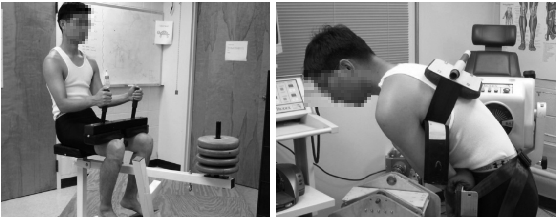
Figure 3.3: Fatiguing exercise were performed with a seated calf raise device for ankle plantar flexor fatigue (left), and with a custom attachment designed for the Biodex System 3 Pro dynamometer for lumbar extensor fatigue (right).
