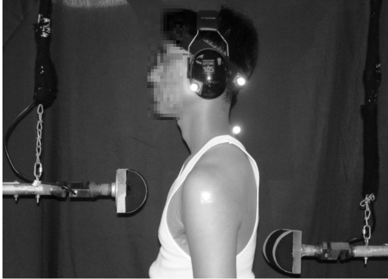
Figure 3.1: Participants were perturbed in the anterior and posterior directions with padded and weighted ballistic pendulums. Perturbations were administered by pulling the pendulums away from the participant and releasing one from a fixed location to yield the desired perturbation magnitude.(photo by Bradley Davidson)
