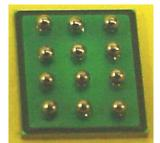
Figure 1.12. Die-dimensional BGA power packages developed in CPES [10].
