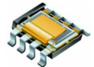
Figure 1.14. A chip-level CopperStrap power package [14].
