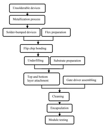
Fig. 2 The FCOF-IPEM fabrication flowchart.
