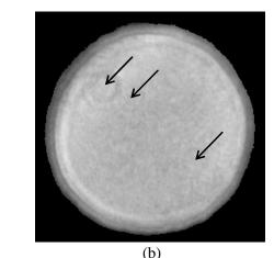
Fig. 4. SAM images of the solder/copper interface in the bi-layered specimens #4 (a) and #5 (b), respectively. Both specimens have a diameter of 1.27 cm. Arrows in (b) indicate the low density areas at the solder/copper interface.
