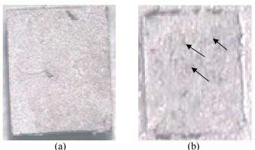
Figure 3.41. Optical microscopy pictures of one of the sheared-off Infineon SiC device (a) and the corresponding die-attach cavity on the gold-coated DBC substrate (b). The arrows in (b) indicate the debonding areas from the gold-silver interface.
