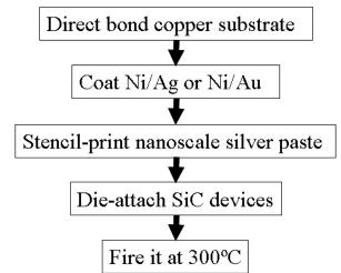
Figure 2.21. Preparation steps of the sintered sliver joint samples.
