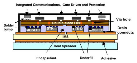
Fig. 1. Schematic structure of an FCOF-IPEM built using solder-bumped power devices.
