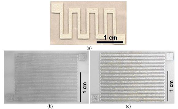
Figure 3.8. Screen-printed and low-temperature sintered silver patterns on alumina substrates.
