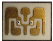
Figure 4.16. Low-temperature sintered silver die-attached LEDs. The two white parts are dispensed-silver after low-temperature sintering and the two blacks squares are two die-attached LEDs.
