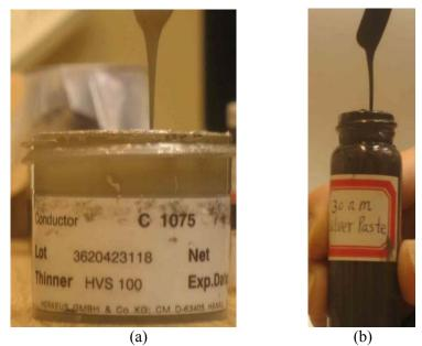
Figure 3.2. Good flowability of the commercial microscale silver paste (a) and that of the 78 wt.% nanoscale silver paste.
