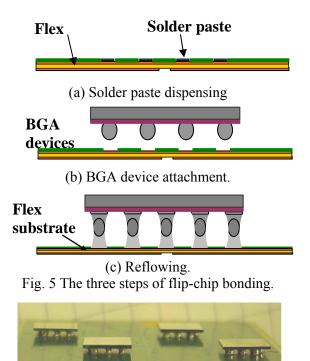
Fig. 6 The power devices and flex substrate assembly after flip-chip bonding.
