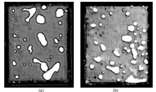
Figure 1.26. The initial void problems in the reflowed die-attaching solder layers in (a) lead-tin solder and (b) lead-free solder.
