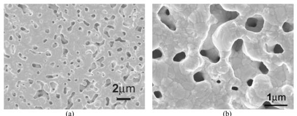
Figure 3.11. Microstructure of the low-temperature sintered nanoscale silver on an alumina substrate (top surface of a sintered film with thickness about 1 mil). (a) at 10 Kx and (b) 50 Kx.
