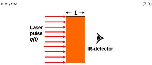
Figure 2.11. Illustration of the laser-flash experiment.
