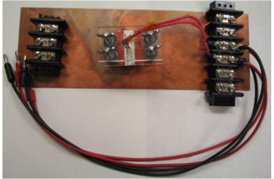
Figure 2.27. Fixture for the high-power curve tracer tests.
