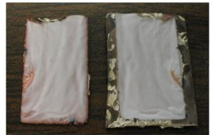
Figure 3.44. An alumina DBC substrate broken from the alumina layer between 100-200 cycles switching from 50°C to 300°C.
