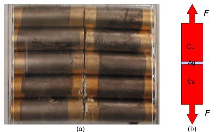
Figure 2.14. Nickel/gold plated copper rods for the preparation of sintered silver joints (a) and their debonding illustration.
