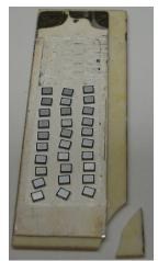
Figure 3.45. Another alumina DBC substrate broken from the alumina layer between 500 to 1000 cycles switching from 50°C to 250°C.
