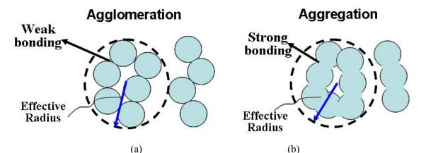
Figure 1.21. Illustration of agglomeration (a) and aggregation (b) and their effective particle sizes.
