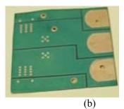
Fig. 4 A flex substrate which has a simple gate driver circuit on one side (a) and the power stage circuit on the other side (b).
