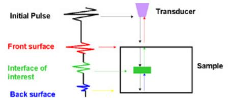
Figure 2.28. The pulse-echo mode illustration in scanning acoustic microscopy.
