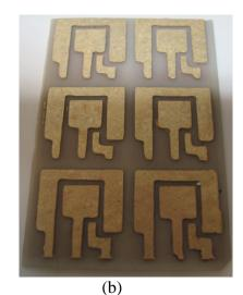
Figure 4.7. The etched and nickel/gold coated DBC substrates for the IXSD35N120A dies (a) and those for the IXSD1765 dies (b).
