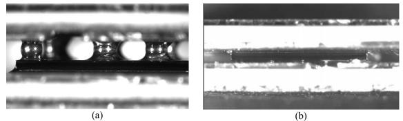
Fig. 1. (a) A SB package with the source/gate of the power MOSFET device attached to the top DBC substrate via six 1-mm-high solder-bumps, (b) a DS package with the source/gate of the device attached to the top DBC substrates via 100 µm solder layers. Both 10X magnification.
