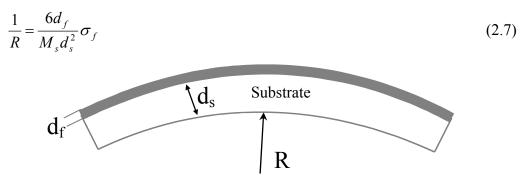
Figure 2.16. Deformation of a film-substrate bilayer composite.
