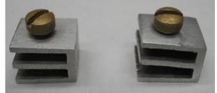
Figure 2.8. Two electrodes used for the measurement of electrical resistance.
