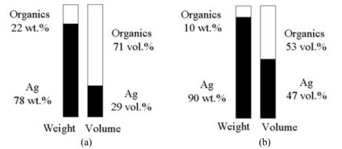
Figure 2.5. The weight and volume percentages of the 78 wt.% silver paste (a) and those of the 90 wt.% silver paste (b).
