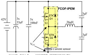
S1&S2: BGA Power MOSFET (IXFD80N08-70) STK D1&D2: BGA Schottky Diode (C-DWS 32-100)
