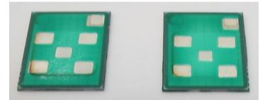
Figure 4.6. The IXSD1765 bare dies after the solder mask deposition to protect the exposed gate fingers. Note that the IXSD1765 dies are already metallized nickel/silver at the open windows for the gate and source terminals.
