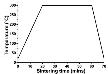
Figure 2.25. The sintering profile for achieve high bonding strength in the silver joints.
