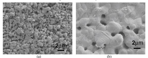
Figure 3.16. The microstructure evolution of the microscale silver paste before (a) and after (b) the heat treatment during the electrical resistivity measurement.
