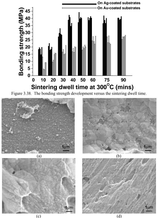
Figure 3.39. Microstructures of the debonded sintered silver joints on the silver-coated SiC devices after dwelling sintering at 300°C for (a) 10 mins, (b) 20mins, (c) 40mins, and (d) 60 mins.
