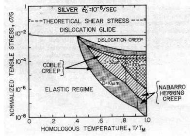
Figure 3.57. The deformation-mechanism map for pure silver, established for a critical strain rate of  $10^{-8}$  s<sup>-1</sup>; it can be seen how the deformation-mechanism fields are affected by the grain size (reprinted from Ref. [12], p.677).
