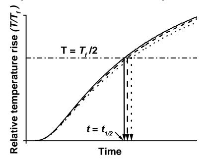
Fig. 2. The changes of the temperature transient curve at the rear surface of a specimen when changing the values of the solder/copper interfacial thermal resistance.
