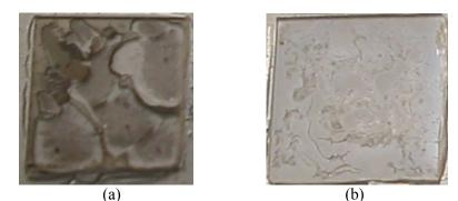
Figure 3.30. The 78 wt.% (a) and 84 wt.% (b) silver paste sintering under the 4×4 mm<sup>2</sup> glass slide coverage after 10-min dwell sintering at 300°C.
