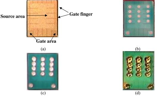
Fig. 3 (a) A commercial unsolderable power MOSFET from IXYS. (b) The MOSFET after solder-mask process. Except the gate and source pads, the entire surface is covered by solder mask. (c) The MOSFET after UBM sputtering process. (d) The solder-bumped MOSFET.
