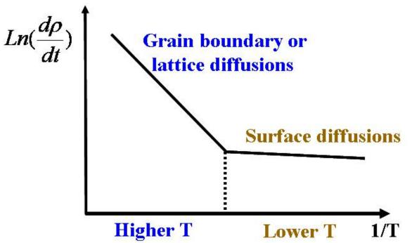
Figure 1.23. Schematic diagram of change in densification rate with temperature. According to rapid rate sintering theory, the two regimes should corresponding to poor or no densification (surface) at low temperatures and much more efficient densification (via grain boundary or lattice diffusion) at high temperature [51].
