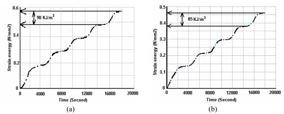
Fig. 11. The average inelastic strain energy density accumulation at the corner elements of the SB (a) and DS (b) interconnections, respectively, during the first five power cycles.
