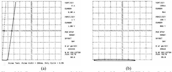
Figure 3.35. Forward (a) and reverse (b) I-V curves obtained from the CREE devices. Dashed curve in (a) is due to the test fixture.
