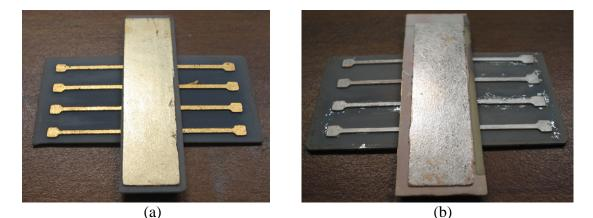
Figure 4.10. The finished single-chip power packages for the IXSD35N120A devices (a) using the nickel-gold plated DBC substrates and (b) the nickel-silver plated DBC substrates.
