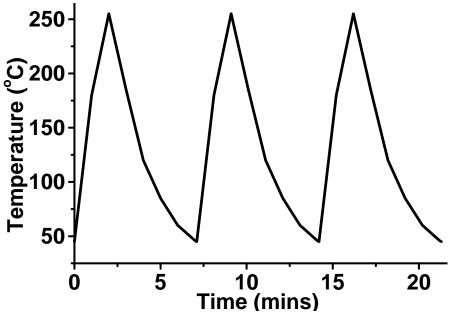
Figure 3.46. The temperature profile obtained using the Sikama belt reflow oven.
