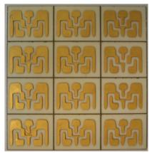
Figure A.2. The etched aluminum oxide DBC substrate for packaging white LEDs.
