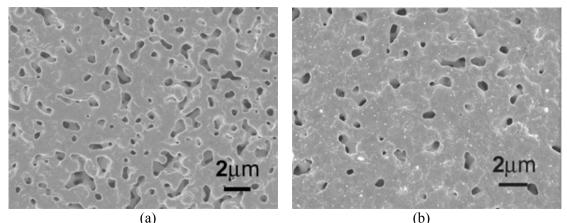
Figure 3.15. The microstructure evolution of the nano-silver paste before (a) and after (b) the heat treatment during the electrical resistivity measurement.
