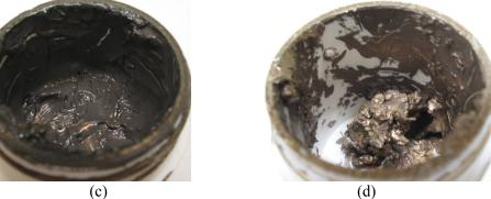
Figure 3.1. The 78 wt.% (a), 84 wt.% (c), and 90 wt.%(d) silver-loading nano- pastes stored in containers. (b) The 78 wt.% silver paste stored in a plastic syringe.
