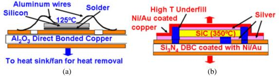
Figure 4.1. The solder die-attaching and wire-bonding technology (a) versus the low-temperature silver sintering technology (b).
