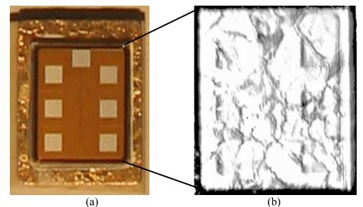
Figure 3.29. The silver sintering die-attached power IGBT with a size of  $8.91 \times 7.22 \text{ mm}^2$  (a) and its SAM image (b).
