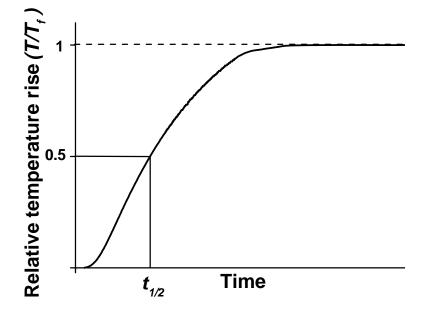
Fig. 1. A typical temperature transient curve at the rear surface of a specimen after the laser flash.
