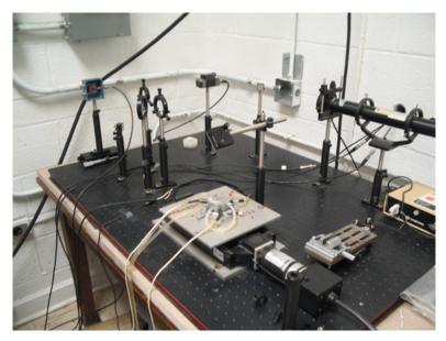
Figure 2.17. The optical setup for measuring the curvature of bi-layer composite during thermal heating.
