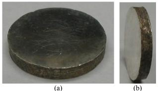
Figure 2.10. The disc-shaped silver specimens prepared by molding and low-temperature sintering.
