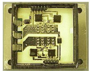
Figure 1.6. An IPEM packaged by the embedded power technology [3].
