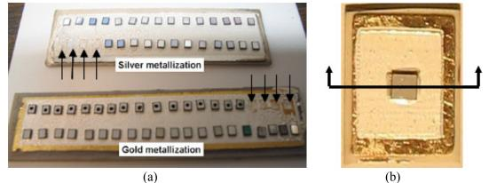
Figure 2.26. (a) Die-attached Infineon SiC devices on silver or gold-coated DBC substrates for the die-shear tests. Arrows indicate the die-attaching cavities where the devices have been sheared-off. (b) A die-attached CREE device for the cross-sectional inspections.
