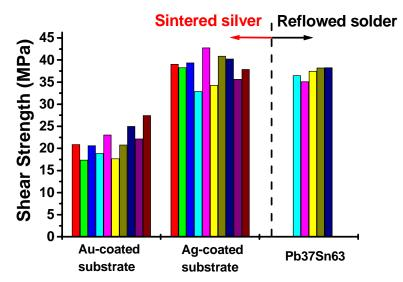
Figure 3.40. The comparison of the shear strength of the low-temperature sintered silver with that of the reflowed solder.
