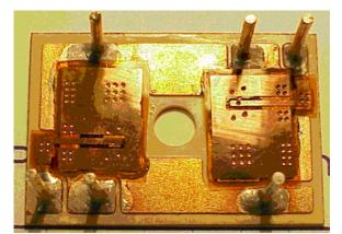
Figure 1.4. A prototype of power module packaged using power overlay interconnect technology.
