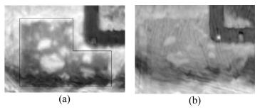
Fig. 6. SAM images of the DS interconnection in a failed DS package taken after 875 thermal cycles. (a) At the solder/power device interface and (b) at the solder/DBC copper interface.
