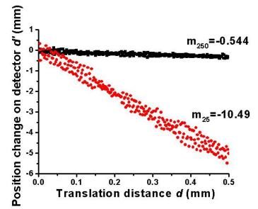
Figure 3.25. The date plot of the position changes in the photodetector versus the scanning distance from the curvature experiment.
