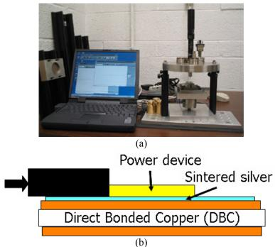
Figure 2.30. The die-shear tester for die-shear-off test (a) and illustration for die shear-off (b).
