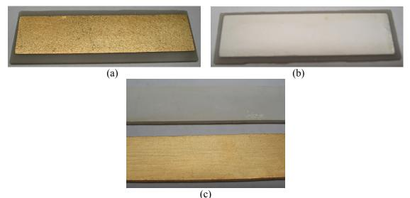
Figure 2.22. Nickel/gold (a) and nickel/silver (b) coated AIN DBC and the nickel/silver and nickel/gold coated copper substrates (c).
