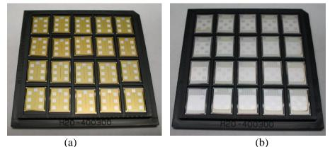
Figure 4.2. The IXYS bare dies used for single-chip power packaging demonstration. (a) Bare power IGBTs with type # of IXSD35N120A; (b) Bare power IGBTs with type # of IXSD1765.
