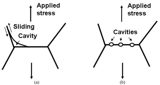
Figure 3.58. *w*-type cavitation at a grain-boundary triple point (a) and *r*-type cavitation at a grain boundary normal to the stress axis (adapted from Ref. [12], pp. 146-147).
