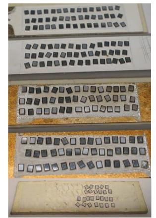
Figure 2.32. The die-attached Infineon SiC devices used for the 50-250°C thermal cycling experiment. From top to bottom: Ag-coated Al<sub>2</sub>O<sub>3</sub> DBC, Ag-coated AlN DBC, Au-coated Al<sub>2</sub>O<sub>3</sub> DBC, Ag-coated AlN DBC, and Ag-coated copper substrates.
