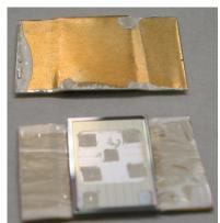
Figure 4.11. The IXSD1765 dies with the drain terminals interconnected to nickel-gold coated copper cavities.
