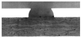
Figure A.1. The over-etch phenomena during the isotropic etching of DBC substrates. For the etching of 0.3 mm DBC Cu layer, the over-etching is about 0.1 mm (100  $\mu$ m).
