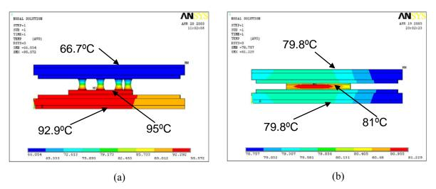
Fig. 7. Thermal FEA temperature distribution results of (a) the SB and (b) the DS packages under the same operation and double-sided cooling conditions.
