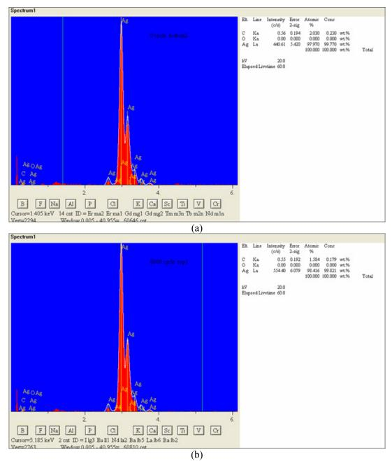
Figure 3.54. EDS analysis of the silver joints before (a) after (b) the 8000 50—250°C thermal cycles. Silver is about 99.8 wt.% and the rest component is carbon. There is no detectable oxygen element before and after thermal cycles.
