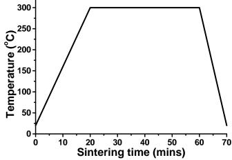
Figure 3.33. The sintering profile for achieving enhanced sintering and high bonding strength for the silver joints with size  $4 \times 4 \text{ mm}^2$  or below.
