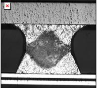
Fig. 7 SEM image of a triple stacked hourglass shaped solder bump.
