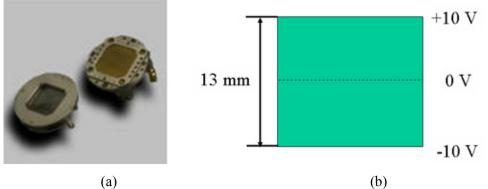
Figure 2.20. The position sensitive photodetectors used in the curvature determination optical setup (a) and their position-sensing mechanism (b).
