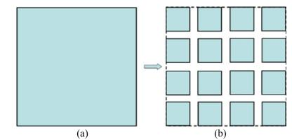
Figure 3.32. Illustration of using small patterns for the enhancement of organic burnout and paste sintering for large area silver bonding.
