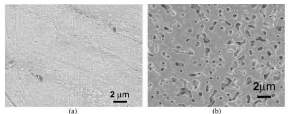
Figure 3.20. Comparison of surface microstructures of the polished samples for the thermal conductivity measurement (a) and those for the electrical conductivity measurement (b) (non-polished).
