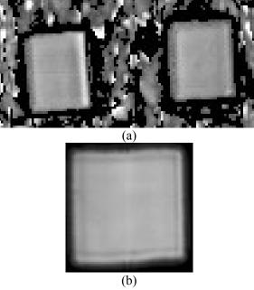
Figure 3.36. SAM images of the sintered silver joints between the SiC devices and the goldcoated DBC substrate. (a) from the Infineon devices measured of  $1.706 \times 1.38 \text{ mm}^2$  and (b) from the CREE devices measured of  $2.26 \times 2.26 \text{ mm}^2$ .
