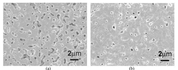
Figure 3.12. Microstructures of the low-temperature sintered nanoscale silver (a) by follows the profile in Figure 2.6 and (b) abrupt sintering, respectively.
