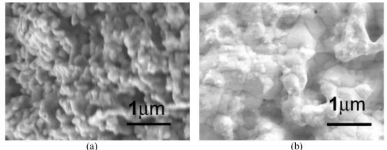
Figure 3.28. The comparison of the microstructures of unsintered silver (a) with those of sintered silver (b).
