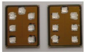
Figure 4.5. The IXSD35N120A bare dies after the sputtering metallization and low-temperature sintering of stencil-printed silver paste on the gate and source terminals. The top middle square is for gate and other six are for the source.
