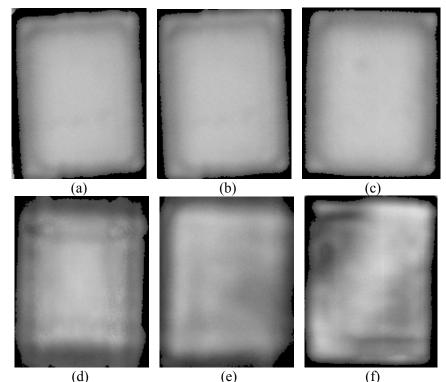
Figure 3.48. SAM images of the sintered silver joints on nickel/gold-coated Al<sub>2</sub>O<sub>3</sub> DBC after 0 (a), 1000 (b), 2000 (c), 4000 (d), 6000 (e), and 8000 (f) thermal cycles, respectively.
