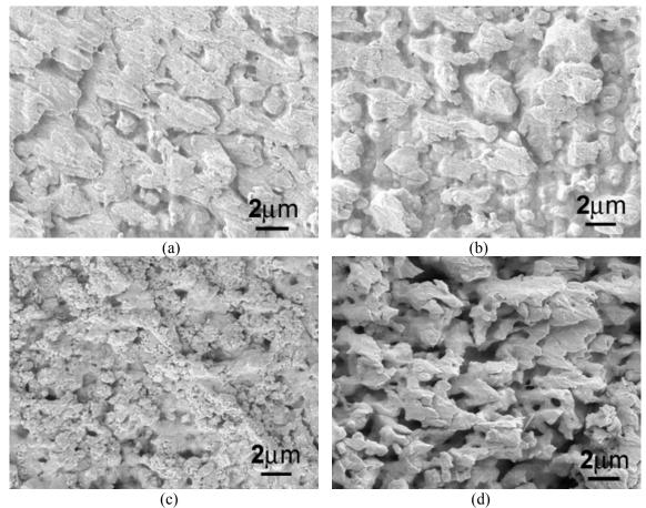
Figure 3.55. Microstructures of the debonded sintered silver joints on the silver-coated SiC devices after (a) 0, (b) 2000, (c) 4000, and (d) 6000 cycles. The silver joints were debonded from the nickel/silver aluminum-nitride DBC substrates.
