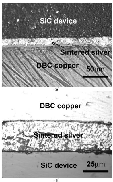
Figure 3.42. Optical microscope pictures of the cross-section of the sintered silver joints.
