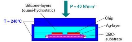
Figure 1.17. Schematic of a pressure-assisted silver paste sintering setup [26].
