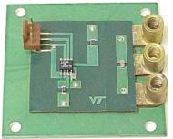
Fig. 9 A completed half-bridge FCOF-IPEM module.
