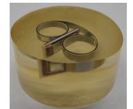
Figure 2.31. A silver joint specimen molded in cured epoxy for polishing and inspection.
