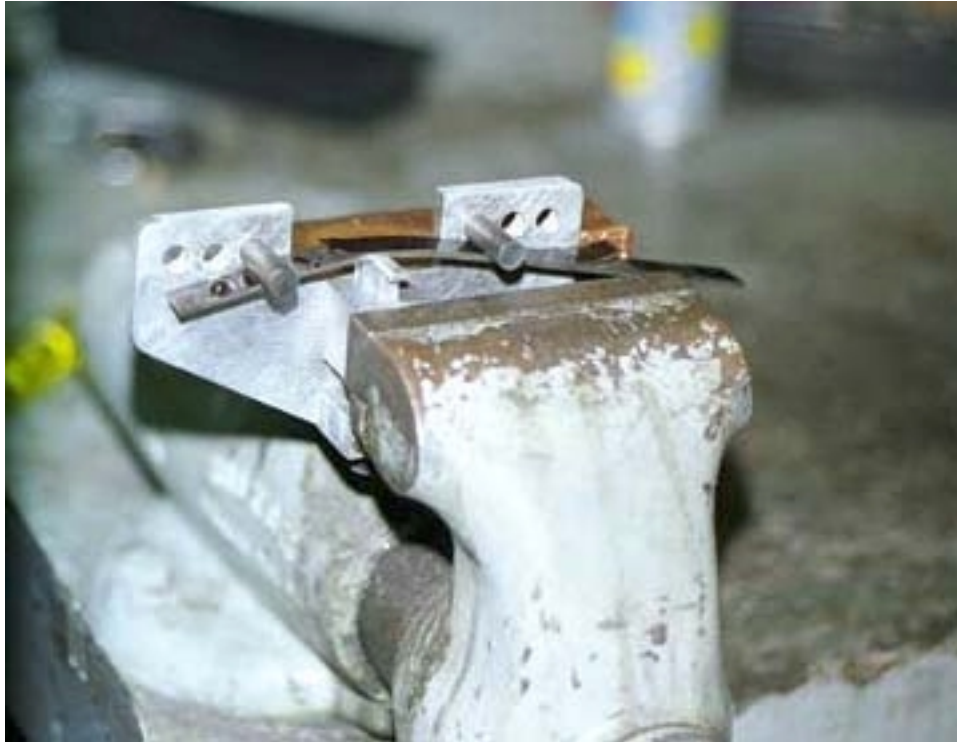
Figure 3.3: Photograph of the three-point bend method used to initiate a debond in the PETI-5 and 8515 NCA specimens.
