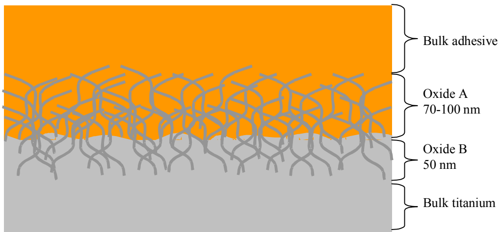
Figure 6.4: Schematic model of the PETI-5/CAA Ti-6Al-4V interphase based on Auger depth profiling data. Oxide A consists of the porous oxide layer embedded with adhesive. Oxide B is the porous oxide layer that contains no adhesive.
