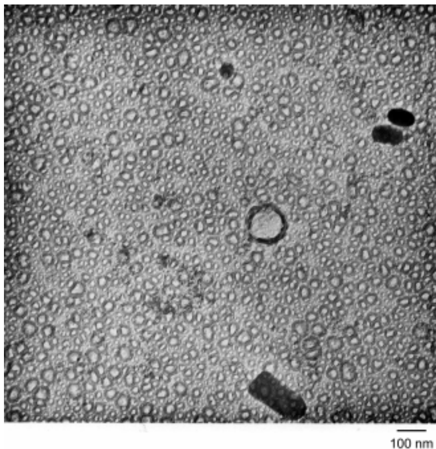
Figure 6.20. Transmission Electron Micrograph of Anodic Film Formed on 6061-T6 in 1 M Ethylphosphonic Acid - 10 V, 5 min, 23°C
