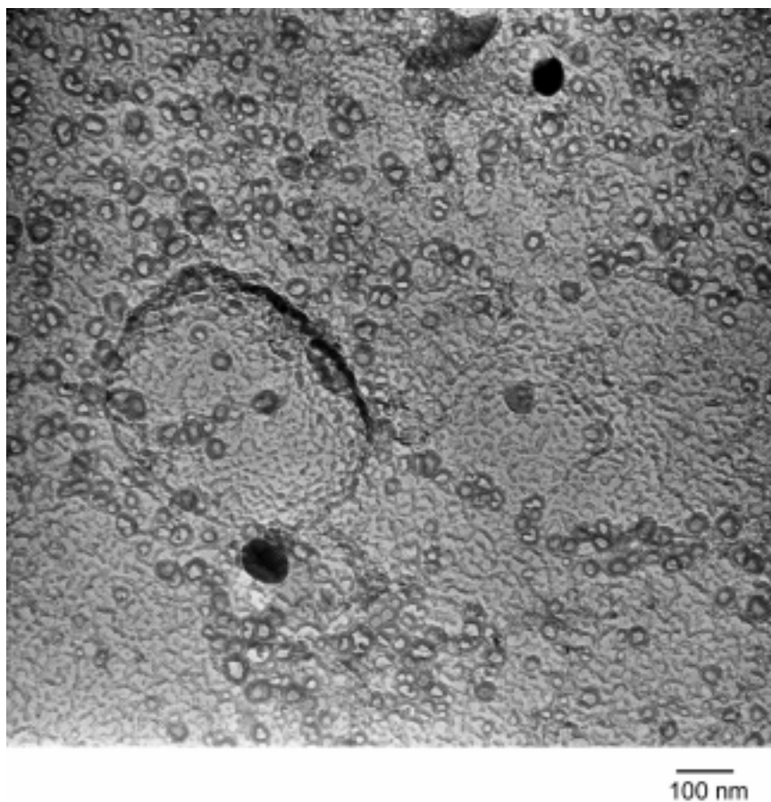
Figure 6.13. Transmission Electron Micrograph of Anodic Film Formed on 6061-T6 in 1 M Vinylphosphonic Acid - 10 V, 5 min, 23°C
